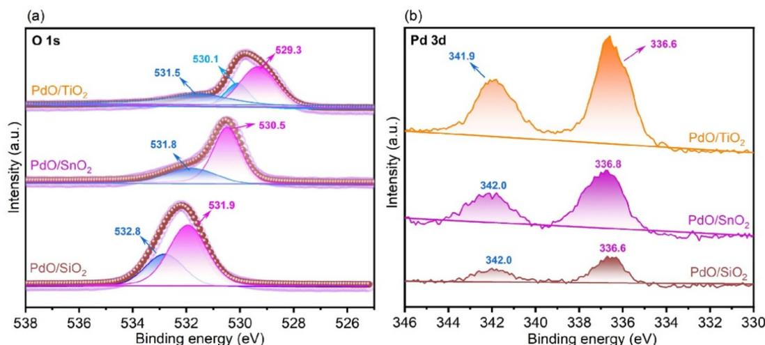
Fig. 5 The XPS spectra of all freshly prepared catalysts are presented as follows: (a) O 1s and (b) Pd 3d XPS spectra of PdO/TiO<sub>2</sub>, PdO/SnO<sub>2</sub>, and PdO/SiO<sub>2</sub>.
