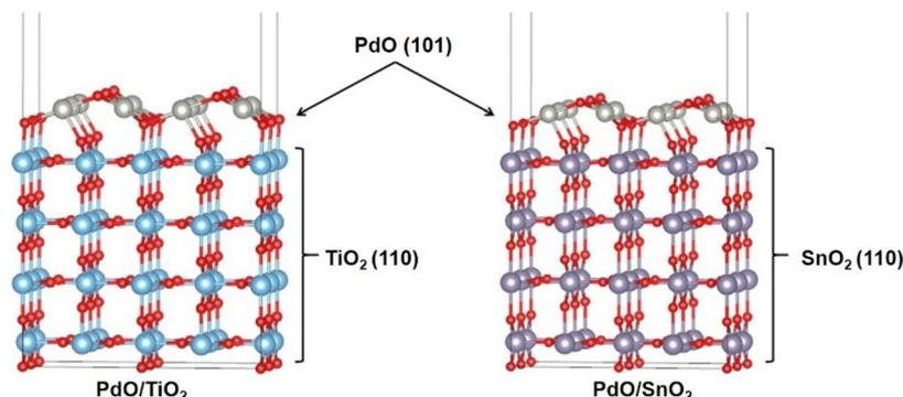
Fig. 1 Model diagrams of the PdO/TiO<sub>2</sub> and PdO/SnO<sub>2</sub> catalysts that were constructed utilizing VASP software by application of the DFT-D3 method.
