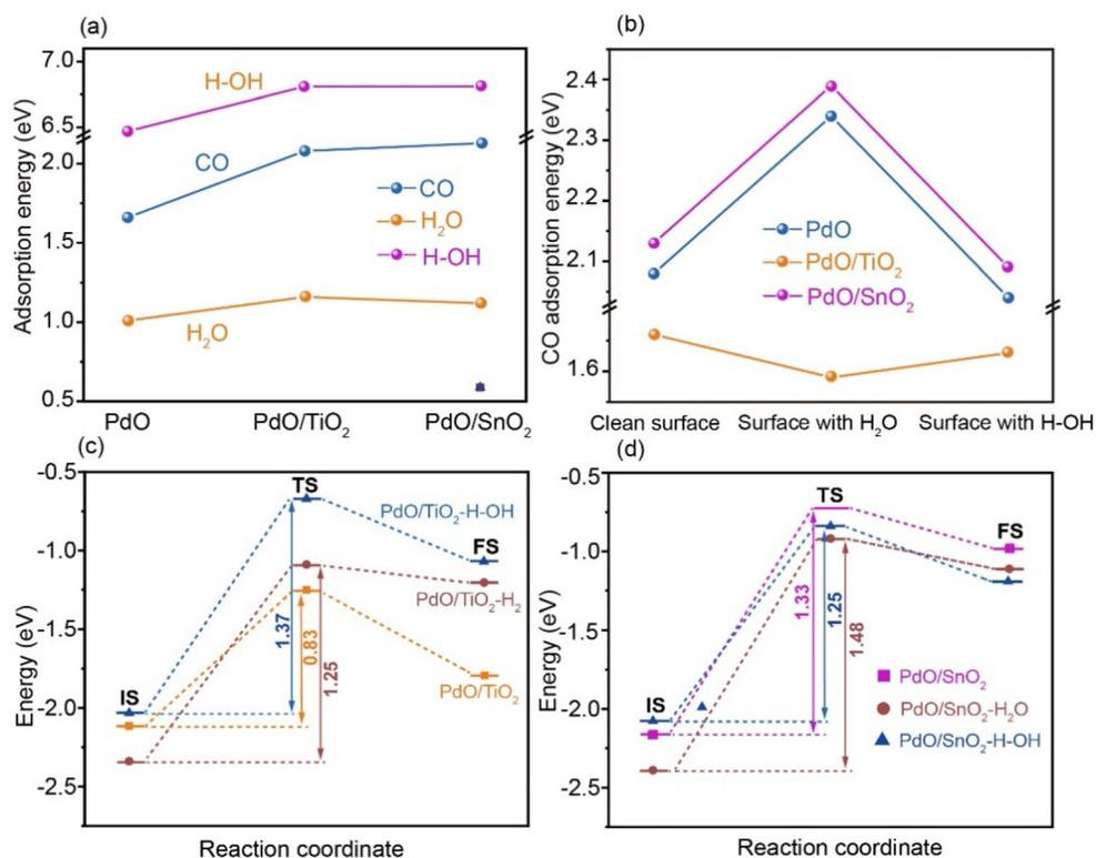
**Fig. 7** (a) Adsorption of small molecules on catalyst surfaces, (b) CO adsorption on catalyst surfaces under different conditions, (c) PdO/TiO<sub>2</sub> and (d) PdO/SnO<sub>2</sub>, and the potential energy diagram for CO oxidation on the surface of catalysts.
