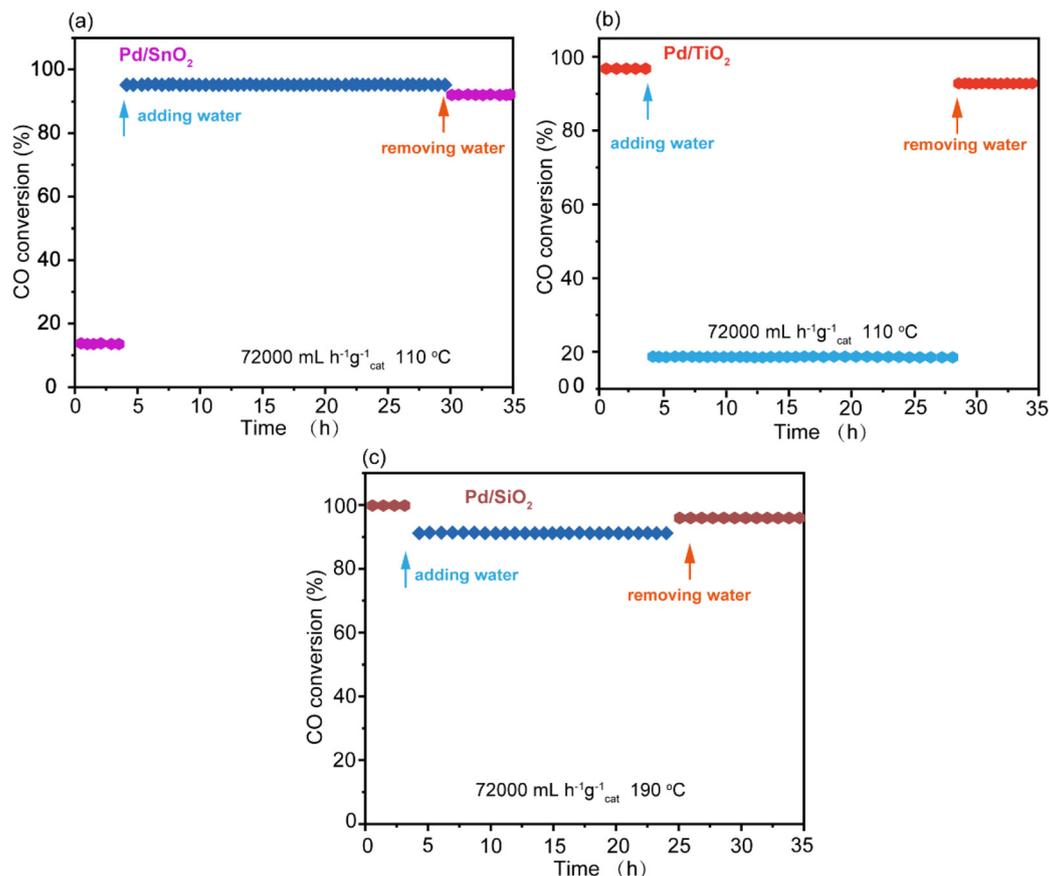
**Fig. 4** Stability test of the CO oxidation reaction on catalyst surfaces in the presence of H<sub>2</sub>O: (a) Pd/SnO<sub>2</sub>, (b) Pd/TiO<sub>2</sub>, and (c) Pd/SiO<sub>2</sub>. Reaction conditions: 1 bar, with a weight hourly space velocity (WHSV) of 72 000 mL g<sup>-1</sup> h<sup>-1</sup>.
