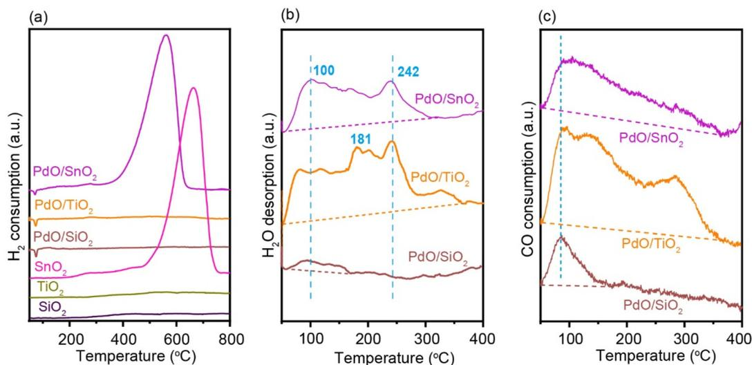
Fig. 6 Characterization of (a) H<sub>2</sub>O-TPR, (b) H<sub>2</sub>O-TPD and (c) CO-TPD of all catalysts.
