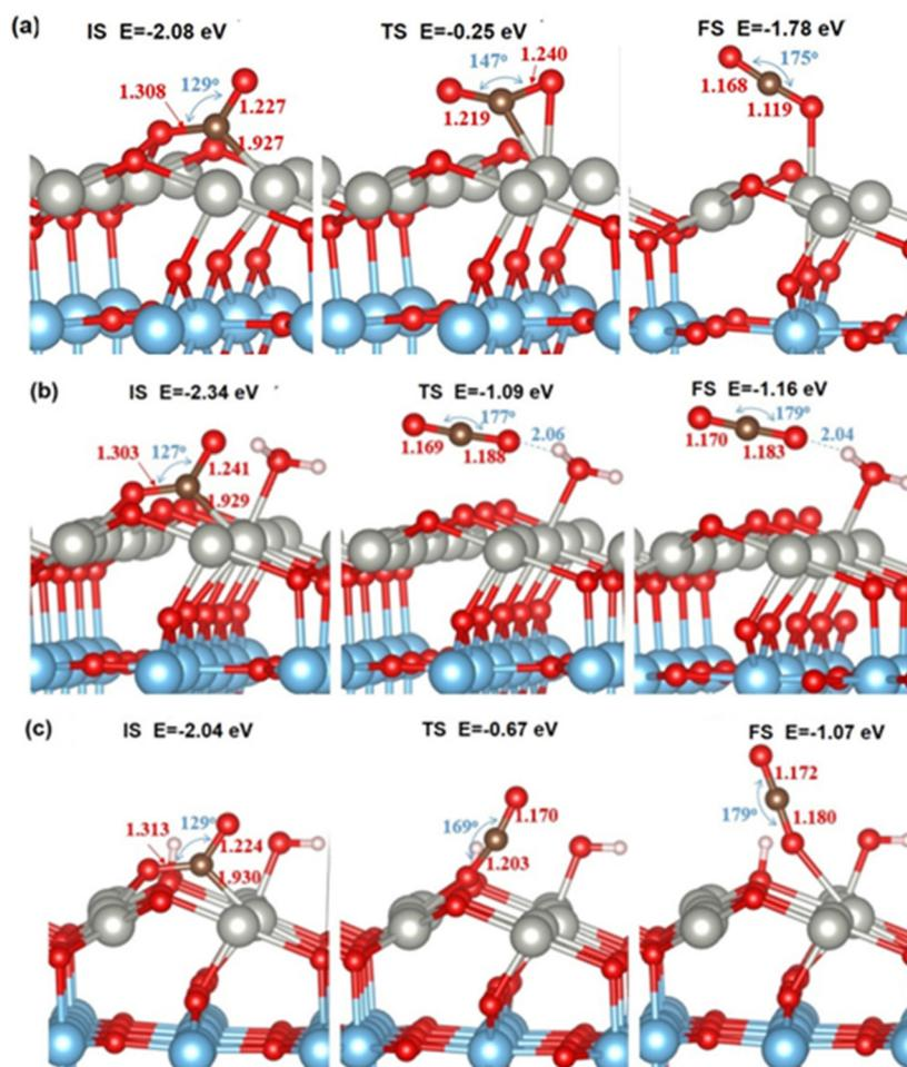
Fig. 8 Surface CO oxidation configuration of PdO/TiO<sub>2</sub> in the absence and presence of water. The energy parameters for the (a) initial (IS), (b) transition (TS), and (c) final states (FS) of the catalyst configuration.
