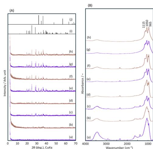
**Fig. 3** (A) XRD patterns and (B) FT-IR spectra of calcined BNDHP<sup>-</sup>/LZH (pH 5.0, 60 °C), respectively: (a, c, e, and f) *R*-BNDHP<sup>-</sup>/LZH, (b, d, f, and h) *S*-BNDHP<sup>-</sup>/LZH. Calcination temperature (°C): (a and b) 500 °C; (c and d) 600 °C; (e and f) 700 °C; (g and h) 800 °C. (i) and (j) assigned to  $\alpha$ -Zn<sub>3</sub>(PO<sub>4</sub>)<sub>2</sub> (JCPDS #29-1390) and ZnO (JCPDS #36-1451), respectively.
