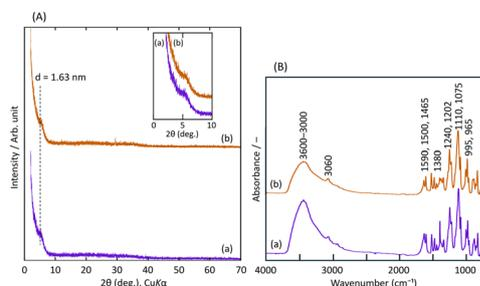
**Fig. 1** (A) XRD patterns and (B) FT-IR spectra of BNDHP<sup>–</sup>/LZH, respectively: (a) *R*-BNDHP<sup>–</sup>/LZH (pH 5.0, 60 °C), and (b) *S*-BNDHP<sup>–</sup>/LZH (pH 5.0, 60 °C). The inset of (A) shows an expanded view of XRD patterns in the low-angle region ( $2\theta = 0–10^\circ$ ).
