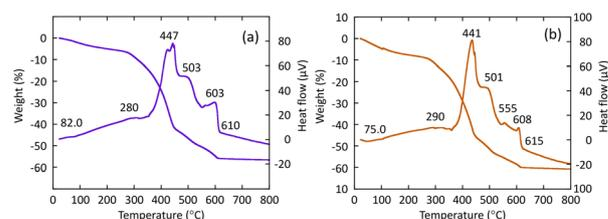
**Fig. 2** TG/DTA curves of BNDHP<sup>–</sup>/LZH, respectively: (a) *R*-BNDHP<sup>–</sup>/LZH (pH 5.0, 60 °C) and (b) *S*-BNDHP<sup>–</sup>/LZH (pH 5.0, 60 °C).
