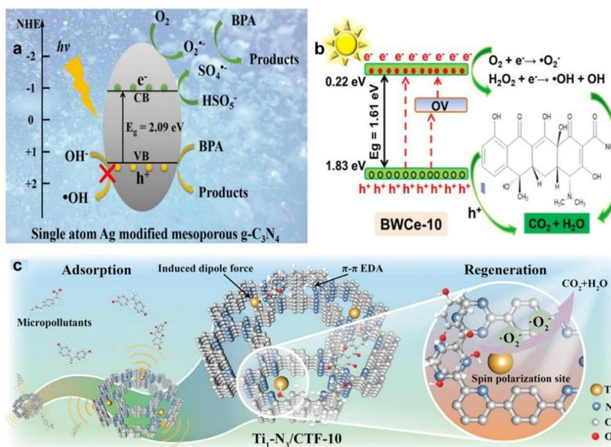
**Fig. 10** (a) Schematic of photocatalytic degradation pathway on single atom Ag-modified mesoporous g-C<sub>3</sub>N<sub>4</sub>. Reproduced with permission.<sup>25</sup> Copyright 2017, Elsevier. (b) Photocatalytic mechanism of the BWCe-10 photocatalyst for TCH degradation. Reproduced with permission.<sup>92</sup> Copyright 2024, American Chemical Society. (c) Schematic diagram of the mechanism for removing pollutants. Reproduced with permission.<sup>93</sup> Copyright 2023, Wiley-VCH.
