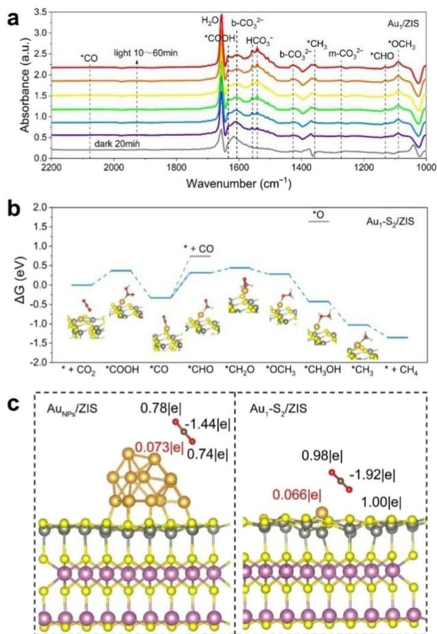
**Fig. 6** (a) Detecting intermediates in reactions *via in situ* DRIFTS, (b) free energy diagram for the conversion of CO<sub>2</sub> to CH<sub>4</sub>, (c) the optimized adsorption arrangements of CO<sub>2</sub> molecules with their associated charge distribution on the surface of AuNPs/ZIS and Au<sub>1</sub>-S<sub>2</sub>/ZIS. Reproduced with permission.<sup>39</sup> Copyright 2022, Wiley-VCH.
