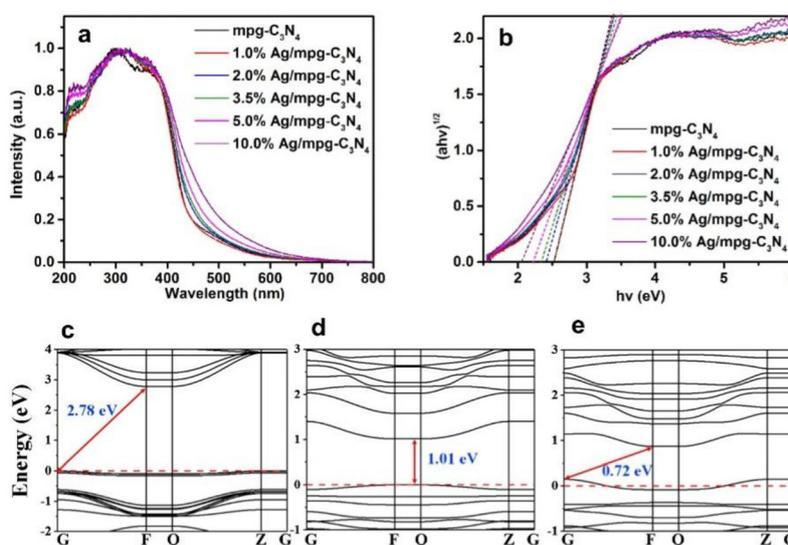
Fig. 2 The UV-vis diffuse reflectance spectra (a) Tauc plots (b) of Ag/mpg-C<sub>3</sub>N<sub>4</sub> with varying Ag loading amounts. Reproduced with permission.<sup>25</sup> Copyright 2017, Elsevier. The energy band structures of (c) pristine g-C<sub>3</sub>N<sub>4</sub>, (d) Fe/g-C<sub>3</sub>N<sub>4</sub>, and (e) Co/g-C<sub>3</sub>N<sub>4</sub>. Reproduced with permission.<sup>55</sup> Copyright 2018, Elsevier.
