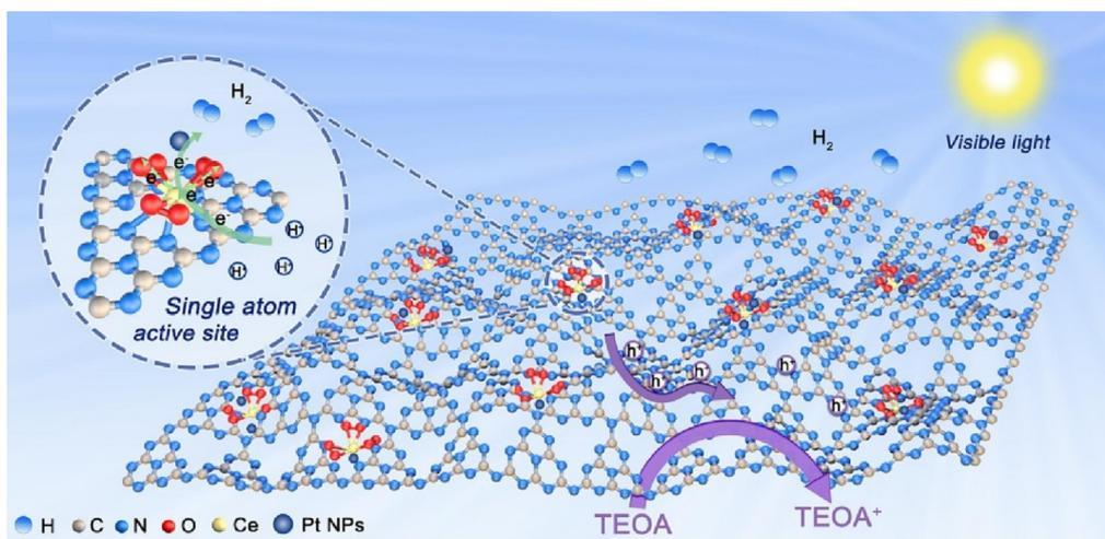
**Fig. 8** The illustrative representation of the photocatalytic hydrogen generation process in Ce-SA-C<sub>3</sub>N<sub>4</sub>. Reproduced with permission.<sup>26</sup> Copyright 2023, Elsevier.
