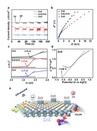
Fig. 4 (a) Piezo-current response of different catalysts; (b) EIS Nyquist plots of the samples; (c) Tauc plots of the samples; (d) Mott-Schottky plot of ZnS; (e) proposed reaction mechanism for piezocatalytic H<sub>2</sub> production over ZnS-ZnO composite nanosheets.
