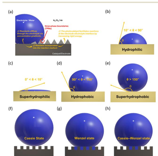
**Fig. 1** Schematic of (a) three-phase contact line where the electrolyte–water droplet meets the solid surface and the surrounding gas. Schematic of (b) hydrophilic, (c) superhydrophilic, (d) hydrophobic, and (e) superhydrophobic surfaces with different wetting/non-wetting states. Reprinted (adapted) with permission.<sup>15</sup> Copyright 2024, Elsevier. Schematic of a liquid drop under (f) Cassie state, (g) Wenzel state, and (h) Cassie–Wenzel state.
