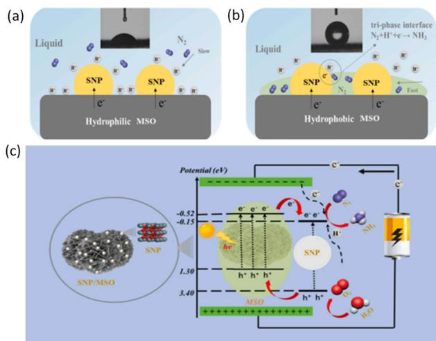
**Fig. 5** Schematic diagram of the three-phase reaction interface of  $N_2$ , electrolyte and catalyst (a) hydrophilic interface and (b) hydrophobic interface. (c) Schematic diagram of the SNP/MSO heterostructure PEC NRR mechanism. Reprinted (adapted) with permission.<sup>119</sup> Copyright 2022, Elsevier.
