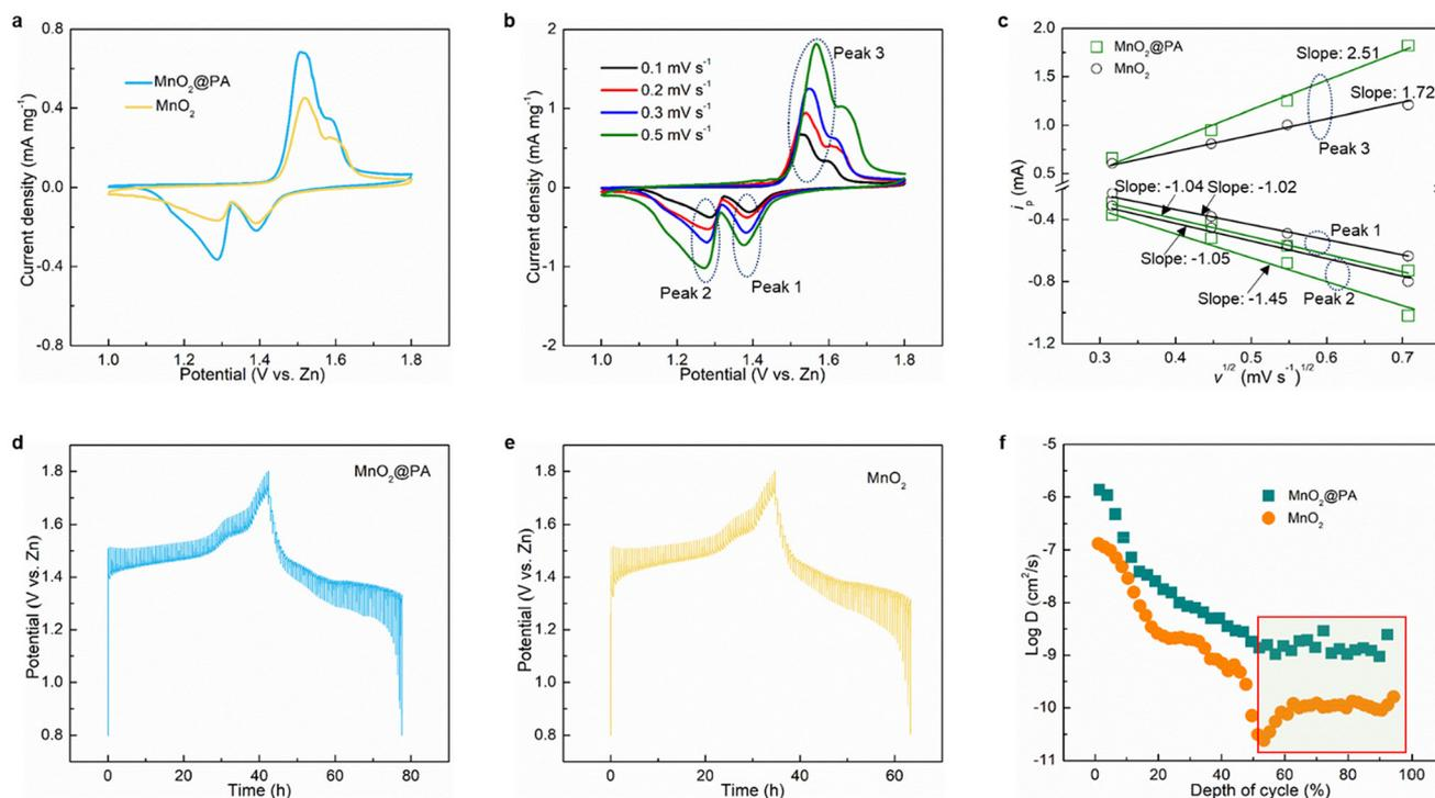
**Fig. 4** Electrochemical reaction kinetics of different cathodes. (a) CV curves for MnO<sub>2</sub> and MnO<sub>2</sub>@PA. (b) CV curves of MnO<sub>2</sub>@PA at various sweep rates. (c) The dependence of log (peak current) on log (scan rate) for obtaining *b* values. Charge/discharge profiles of (d) MnO<sub>2</sub>@PA and (e) MnO<sub>2</sub> during the GITT measurements. (f) The ion diffusion coefficient vs. voltage for MnO<sub>2</sub>@PA and MnO<sub>2</sub> during the 2nd discharge.
