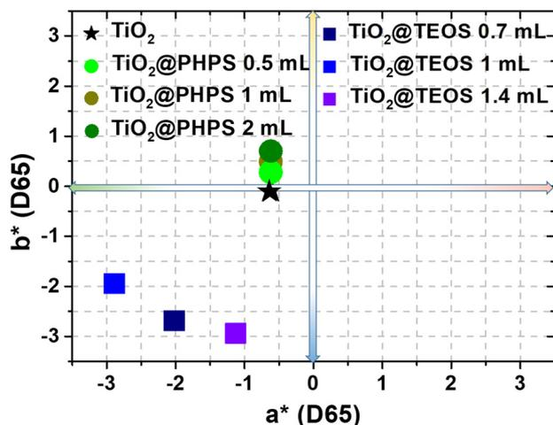
Fig. 4 CIE *a\*b\** chromaticity diagram of whiteness parameters of the TiO<sub>2</sub>, TiO<sub>2</sub>@TEOS, and TiO<sub>2</sub>@PHPS core-shell nanoparticles fabricated in this study with different TEOS and PHPS precursor concentrations.
