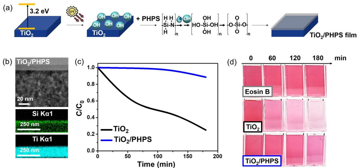
**Fig. 5** (a) Schematic representation of the TiO<sub>2</sub>/PHPS film prepared *via* 'self-catalysed method'. (b) Cross-sectional TEM images of the TiO<sub>2</sub>/PHPS thin film. (c) Photocatalytic degradation of Eosin B as a function of time by the TiO<sub>2</sub> and TiO<sub>2</sub>/PHPS thin films. (d) Camera-captured images of the Eosin B solution following its photocatalytic degradation by the TiO<sub>2</sub> and TiO<sub>2</sub>/PHPS films under UV-A irradiation.
