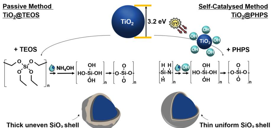
**Fig. 1** Schematic representation of the  $\text{TiO}_2@TEOS$  core-shell nanoparticles prepared via 'passive method', and the  $\text{TiO}_2@PHPS$  core-shell nanoparticles prepared via 'self-catalysed method'.
