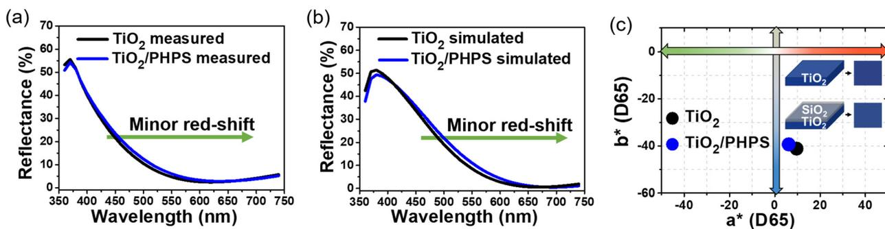
**Fig. 6** (a) Measured and (b) simulated reflectance spectra of TiO<sub>2</sub> and TiO<sub>2</sub>/PHPS films. (c) CIE a\*b\* chromaticity diagram of colour parameters of the TiO<sub>2</sub> and TiO<sub>2</sub>/PHPS films. Insert in top right corner illustrates measured colours and their corresponding films.
