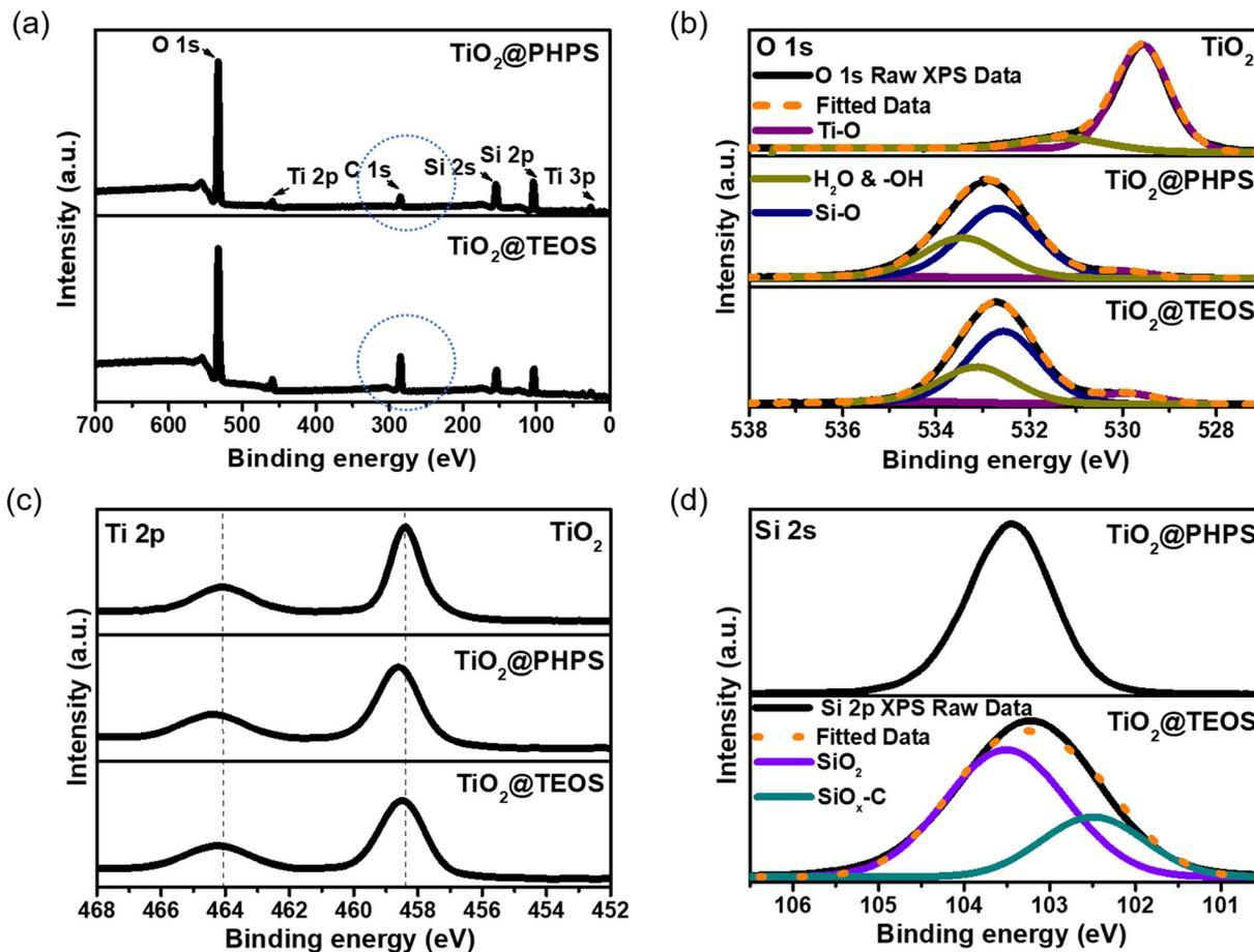
Fig. 2 (a) Full scan survey XPS spectra of 0.7 mL  $\text{TiO}_2$ @TEOS and 1 mL 3 h irradiated  $\text{TiO}_2$ @PHPS core-shell nanoparticles. Narrow-scan XPS spectra of (b) deconvoluted O 1s, (c) Ti 2p, and (d) deconvoluted Si 2p binding energy ranges of the  $\text{TiO}_2$ ,  $\text{TiO}_2$ @TEOS, and  $\text{TiO}_2$ @PHPS core-shell nanoparticles.
