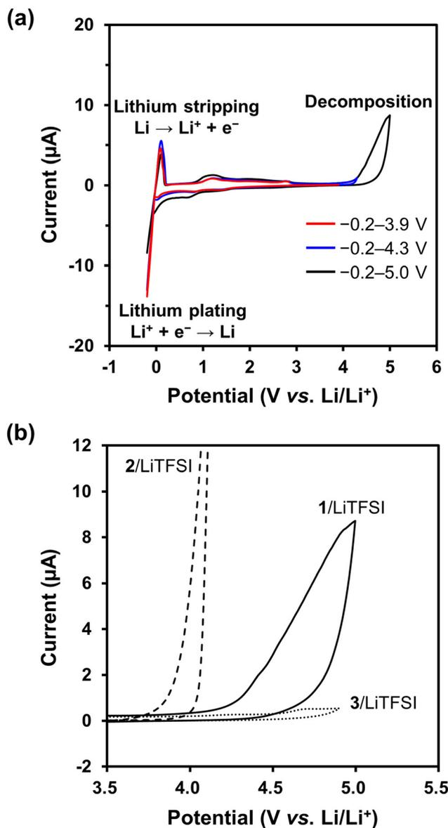
**Fig. 9** (a) Cyclic voltammograms of the LC electrolyte **1**/LiTFSI at an 80 : 20 molar ratio in the voltage region of -0.2–3.9 V (red), -0.2–4.3 V (blue), and -0.2–5.0 V (black) vs. Li/Li<sup>+</sup> at 60 °C. (b) Enlarged CV curves in the high voltage region of **1**/LiTFSI at an 80 : 20 molar ratio (black solid line), **2**/LiTFSI at a 90 : 10 molar ratio<sup>12</sup> (black dashed line), and **3**/LiTFSI at an 80 : 20 molar ratio<sup>12</sup> (black dotted line).
