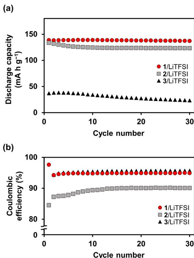
Fig. 11 Cycling performance of half-cells of Li/LC electrolytes/LiFePO<sub>4</sub> using 1/LiTFSI at an 80 : 20 molar ratio (red circle), 2/LiTFSI at a 90 : 10 molar ratio<sup>11,12</sup> (grey square), and 3/LiTFSI at an 80 : 20 molar ratio<sup>12</sup> (black triangle) at 60 °C. Potential range: 2.5–3.9 V for 1/LiTFSI and 2/LiTFSI, and 2.7–3.8 V for 3/LiTFSI; current density: 5 mA g<sup>-1</sup>. (a) Discharge capacity; (b) coulombic efficiency.
