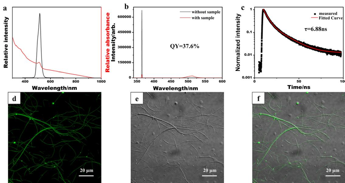
Fig. 3 Optical characterization of CsPbBr<sub>3</sub>/PbSe nanowires: (a) UV/vis absorption and photoluminescence spectra, (b) PLQY, (c) lifetime, (d) confocal fluorescence image, (e) bright field image and (f) merged image of (d) and (e).
