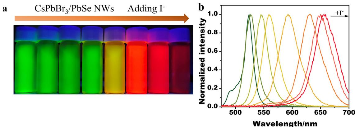
Fig. 4 (a) Photograph of colloidal CsPbBr<sub>3</sub>/PbSe NWs reacting with different concentrations of I<sup>-</sup> ions under a 365 nm UV lamp; (b) corresponding photoluminescence spectra of colloidal CsPbX<sub>3</sub>/PbSe perovskite NWs.
