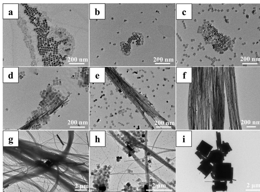
**Fig. 1** TEM images of samples quenched at different times during the transformation from the precursor solution into NWs: (a) 80 °C, (b) 100 °C, (c) 120 °C, (d) 140 °C, (e) 160 °C, 0 min, (f) 160 °C, 20 min, (g) 160 °C, 30 min, (h) 160 °C, 60 min, and (i) 160 °C, 90 min.
