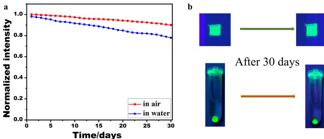
Fig. 5 (a) PL intensity change of colloidal CsPbBr<sub>3</sub>/PbSe NWs in air and in water, (b) photographs of CsPbBr<sub>3</sub>/PbSe NW samples under a 365 nm lamp: top is the CsPbBr<sub>3</sub>/PbSe NWs film on a glass slide exposed to air, and bottom is the centrifuged CsPbBr<sub>3</sub>/PbSe NWs in a tube full of deionized water.
