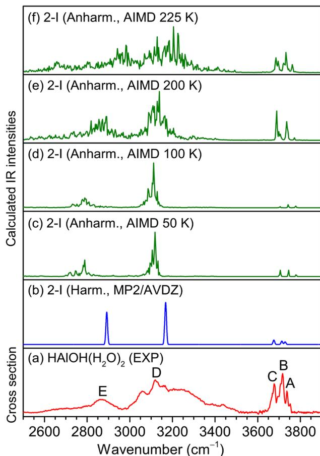
**Fig. 3** Comparison of the experimental IR spectrum of the neutral HAlOH(H<sub>2</sub>O)<sub>2</sub> cluster (a), the MP2/aug-cc-pVDZ calculated harmonic IR spectrum of isomer 2-I (b) and AIMD-simulated anharmonic IR spectra at 50 K, 100 K, 200 K, and 225 K (c–f) of isomer 2-I.
