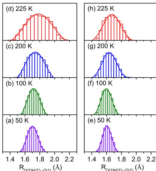
**Fig. 4** Normal distribution of O(2)H(2')...O(1) and O(3)H(3')...O(2) hydrogen-bond distances ( $R_{O(2)H(2')\dots O(1)}$  and  $R_{O(3)H(3')\dots O(2)}$ ) during AIMD simulations of isomer 2-I for HALOH(H<sub>2</sub>O)<sub>2</sub> at 50 K, 100 K, 200 K, and 225 K. The atom labelling is indicated in Fig. 2.
