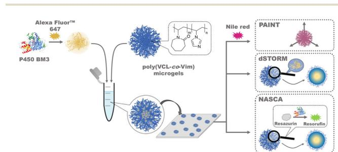
**Fig. 1** Schematic depiction of the experimental set-up for the immobilization of fluorescent labelled P450 BM3 enzymes (crystal structure from PDB: 1BVY) in poly(VCL-*co*-Vim) microgels and their analysis using points accumulation for imaging in nanoscale topography (PAINT), direct stochastic optical reconstruction microscopy (dSTORM), and nanometer accuracy by stochastic chemical reactions (NASCA).
