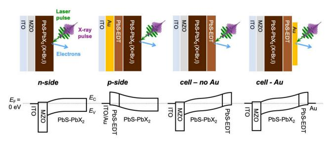
Fig. 1 (Top) Architecture of samples and main elements of a TRPES experiment: X-ray and laser pulses impinging on, and electrons emitted from the sample surface. (Bottom) Band structure illustrations of the different samples based on literature data<sup>4,11</sup> with the Fermi level (E<sub>F</sub>) in the dark indicated by the grey dashed line, the valence band edge  $(E_V)$  indicated as the bottom of the field boxes and the conduction band edge  $(E_C)$  as the top.
