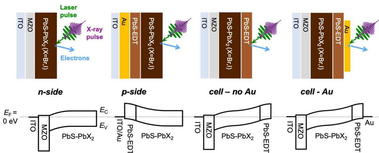
**Fig. 1** (Top) Architecture of samples and main elements of a TRPES experiment: X-ray and laser pulses impinging on, and electrons emitted from the sample surface. (Bottom) Band structure illustrations of the different samples based on literature data<sup>4,11</sup> with the Fermi level ( $E_F$ ) in the dark indicated by the grey dashed line, the valence band edge ( $E_V$ ) indicated as the bottom of the field boxes and the conduction band edge ( $E_C$ ) as the top.
