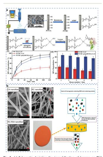
(a) Schematic depicting the immobilization of laccase on PU/ RC-poly(HEMA) nanofiber membrane and its removal efficiency of BPA.<sup>127</sup> Copyright © (2019 and Wiley). (b) Cellulose-based nanofiber membrane functionalized with dye affinity ligand for purification of malate dehydrogenase from Saccharomyces cerevisiae. 132 Copyright © (2022 and Springer).
