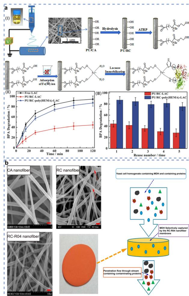
**Fig. 4** (a) Schematic depicting the immobilization of laccase on PU/RC-poly(HEMA) nanofiber membrane and its removal efficiency of BPA.<sup>127</sup> Copyright © (2019 and Wiley). (b) Cellulose-based nanofiber membrane functionalized with dye affinity ligand for purification of malate dehydrogenase from *Saccharomyces cerevisiae*.<sup>132</sup> Copyright © (2022 and Springer).
