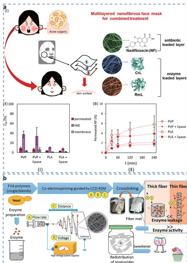
**Fig. 3** (a) The composition of a multilayered nanofibrous face mask for combined treatment of acne vulgaris and investigation of its penetration into human heat-separated epidermis (HSE) applying a topical and transdermal diffusion cell system.<sup>14</sup> Copyright © (2023 and MDPI). (b) Encapsulation of  $\beta$ -glucosidase within PVA fibers to produce specific mogrosidase sweetener.<sup>105</sup> Copyright © (2020 and ACS).
