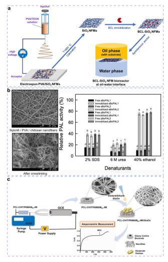
Fig. 2 (a) Construction of BCL-SiO<sub>2</sub> EIEN bioreactor and targeted catalysis at the oil-water interface.<sup>38</sup> Copyright © (2020 and ACS). (b) Images of EIEN nanofibers via cross-linking technique and denaturant tolerance of free and immobilized phenylalanine ammonia-lyases on electrospun nanofibers.84 Copyright © (2021 and MDPI). (c) Glutamate oxidase (GluO<sub>x</sub>)-induced biosensor via covalent binding on electrospun nanofibers.47 Copyright © (2023 and MDPI).
