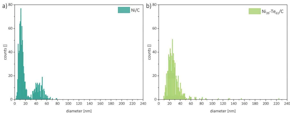
Fig. 5 Particle size distributions of Ni/C (a) and Ni<sub>39</sub>-Te<sub>61</sub>/C (b).
