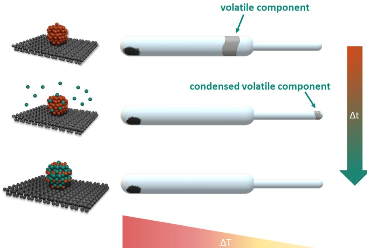
**Fig. 2** Schematic illustration of the vapour–solid synthesis method.
