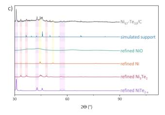
Fig. 3 Measured and refined pXRD patterns with the most significant peaks highlighted of Ni/C (a),  $Ni_{39}$ -Te<sub>61</sub>/C (b) and  $Ni_{67}$ -Te<sub>33</sub>/C (c).
