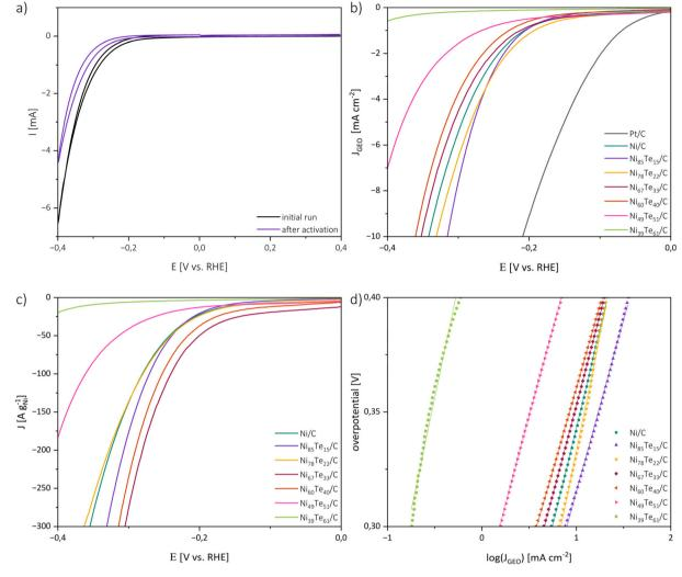
Fig. 6 Cyclic voltammetry curves before and after activation cycling of Ni<sub>85</sub>Te<sub>15</sub>/C (a), polarization curves normalized to the geometric area (b), mass activity normalized to the nickel content (c) and Tafel plots (d).
