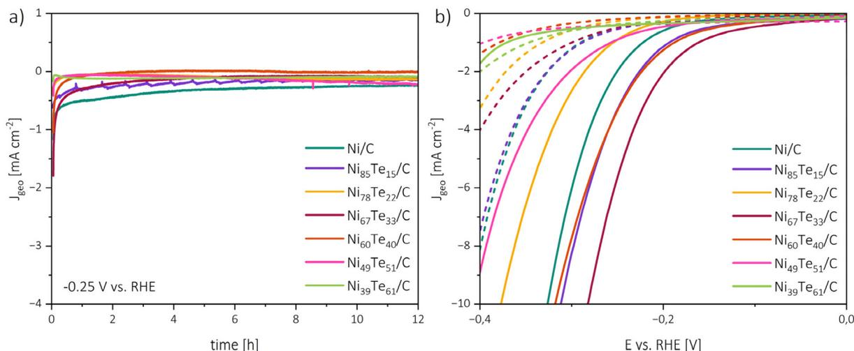
**Fig. 8** Chronoamperometry measurements at  $-0.25 \text{ V vs. RHE}$  and  $1600 \text{ rpm}$  RDE rotation rate (a), polarization curves before chronoamperometry (solid lines) and after chronoamperometry (dashed lines) (b).
