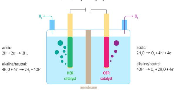
Fig. 1 Scheme of water electrolyser with respective half-cell reactions in acidic, alkaline, and neutral media.
