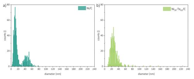
Fig. 5 Particle size distributions of Ni/C (a) and Ni<sub>39</sub>-Te<sub>61</sub>/C (b).
