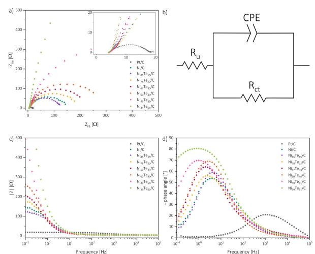
Fig. 7 Nyquist plots (a), modified Randel's circuit ( $R_u$  = uncompensated solution resistance, CPE = constant phase element,  $R_{ct}$  = charge transfer resistance) (b), Bode absolute impedance plot (c) and Bode phase angle plot (d).
