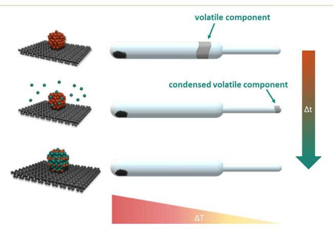
Fig. 2 Schematic illustration of the vapour-solid synthesis method.
