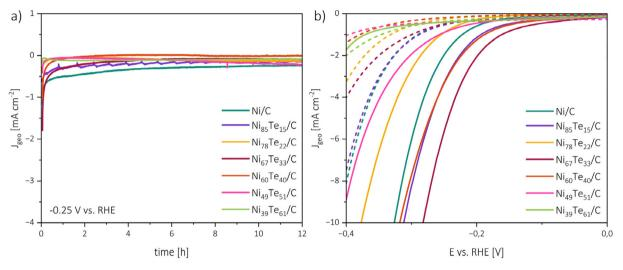
Fig. 8 Chronoamperometry measurements at -0.25 V vs. RHE and 1600 rpm RDE rotation rate (a), polarization curves before chronoamperometry (solid lines) and after chronoamperometry (dashed lines) (b).
