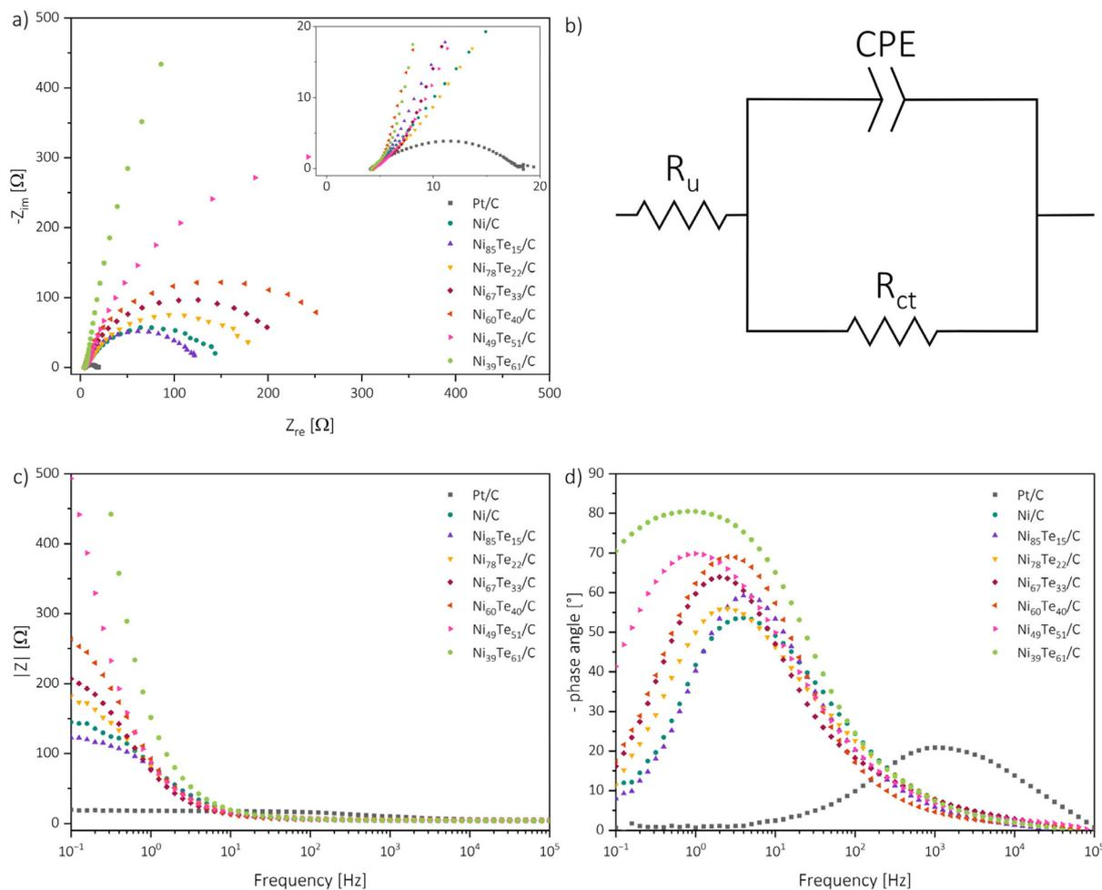
Fig. 7 Nyquist plots (a), modified Randles's circuit ( $R_u$  = uncompensated solution resistance, CPE = constant phase element,  $R_{ct}$  = charge transfer resistance) (b), Bode absolute impedance plot (c) and Bode phase angle plot (d).
