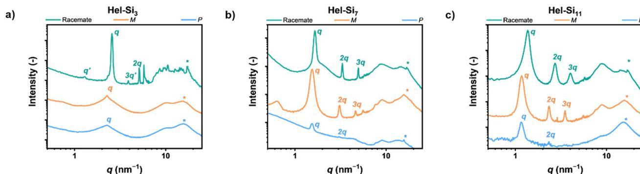
Fig. 3 MAXS/WAXS spectra of the *rac*-, *P*-, and *M*-forms of **Hel-Si<sub>3</sub>** (a), **Hel-Si<sub>7</sub>** (b) and **Hel-Si<sub>11</sub>** (c). It should be noted that the curves of *P*-**Hel-Si<sub>n</sub>** are recorded on Kapton tape due to the small amount synthesized and therefore differences with the enantiomer *M*-**Hel-Si<sub>n</sub>** are observed due to the different processing conditions and the lower sensitivity of the measurement.
