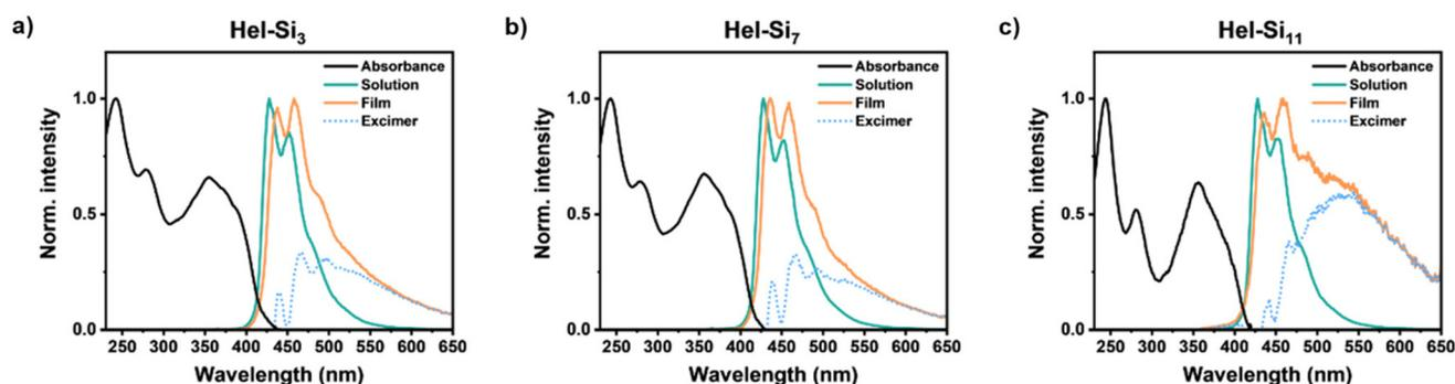
Fig. 5 Absorption and emission spectra of *M*-Hel-Si<sub>*n*</sub> (a, b, and c for *n* = 3, 7 and 11, respectively) in 10<sup>-5</sup> M THF solution and in the solid state recorded as a thin film. The dotted blue trace is the difference between the emission spectra in the solid state and solution to show the excimer. The spectra have all been normalized to unit intensity. The spectra for *P* enantiomers are similar (Fig. S70<sup>†</sup>).
