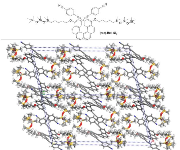
Fig. 4 Chemical structure and supramolecular assembly of 2,15-bis-cyano-phenyl-carbo[6]helicene-siloxane adduct *rac*-Hel-Si<sub>3</sub> obtained from X-ray data analysis.
