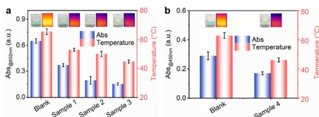
**Fig. 6** Dual-mode TAC detection for skincare products based on the absorption and temperature of CuS@CdS@Au NSs. (a) Absorption intensity at 652 nm and temperature values obtained from different skincare products. (b) Absorption intensity at 450 nm and temperature changes of the sample containing FA.
