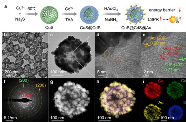
**Fig. 1** (a) Schematic illustration of the synthetic process of CuS@CdS@Au NSs. (b and c) TEM images and (d and e) HR-TEM images of CuS@CdS@Au NSs. (f) SAED pattern of CuS@CdS@Au NSs. (g) HAADF-STEM image of CuS@CdS@Au NSs. (h and i) Elemental mapping images of Cu, Cd, Au, and S in CuS@CdS@Au NSs.
