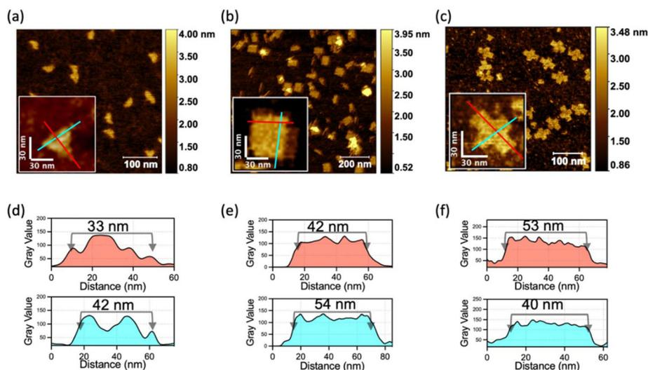
**Fig. 2** Characterization of DNA-assembly structures with different shapes. AFM images of (a) triangle-shaped MUD, (b) rectangle-shaped MUD, and (c) cross-shaped MUD. (d)–(f) Intensity profiles of lines marked in red and cyan corresponding to (a)–(c), which demonstrate the sizes of DNA structures.
