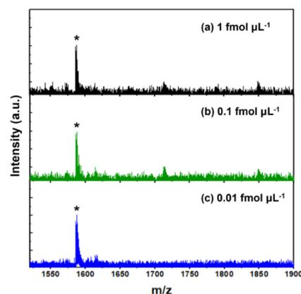
**Fig. 4** Sensitivity evaluation result. MALDI mass spectra of standard peptide (teicoplanin) at different concentrations: (a) 1 fmol μL<sup>−1</sup>, (b) 0.1 fmol μL<sup>−1</sup>, and (c) 0.01 fmol μL<sup>−1</sup>. \* denotes a typical peak of teicoplanin.
