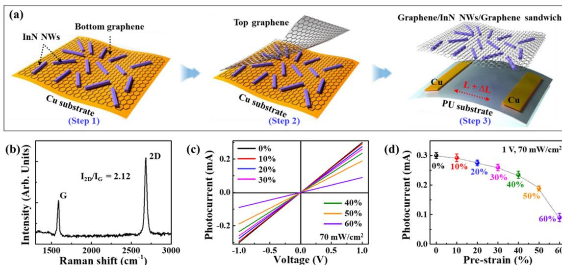
**Fig. 2** (a) Fabrication process of the stretchable photosensor with InN NWs and graphene. (b) Raman spectrum of graphene used as the carrier channel. (c) Characteristic  $I-V$  curves for the stretchable InN-NW photosensors depending on the pre-strain values at the light intensity of  $70 \text{ mW cm}^{-2}$ . (d) Summary of the dependence of the photocurrent on the degree of pre-strain of the PU substrate.
