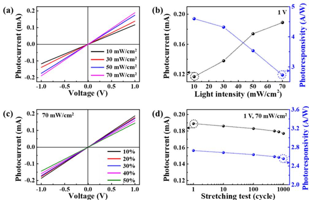
**Fig. 3** (a) Characteristic  $I$ - $V$  curves for the stretchable InN-NW photosensor at various light intensities. (b) Summary of the dependence of the photocurrent and photoresponsivity on the light intensity. (c) Characteristic  $I$ - $V$  curves for the photosensor for the indicated strain values. (d) Summary of the photocurrent of the photosensor for the indicated number of stretching cycles.
