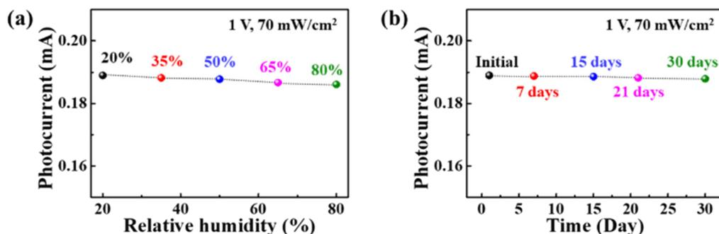
**Fig. 4** (a) Dependence of the photocurrent of the photosensor on the relative humidity. (b) Photocurrent of the photosensor: measured immediately, and 7, 15, 21, and 30 days after device fabrication.
