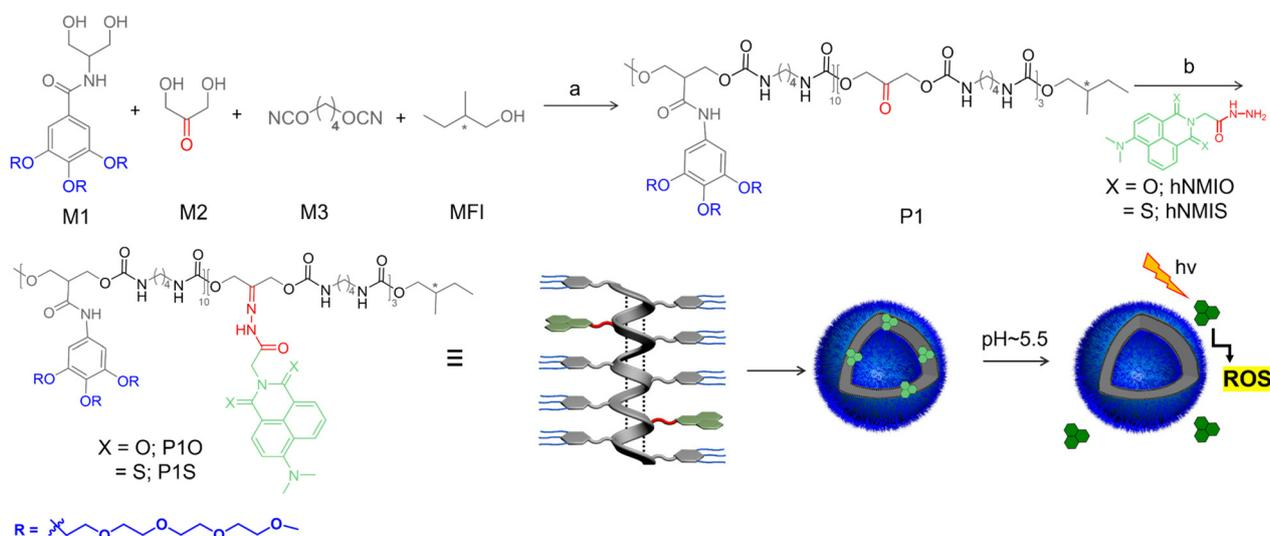
**Scheme 1** Synthesis of activable polymer-photosensitizer conjugate (P1S) and the control polymer (P1O); its chain-folding regulated polymersome assembly and pH-triggered release of the active photosensitizer and ROS generation upon photoirradiation. Reagents and conditions: (a) DABCO, THF, 65 °C, 12 h, 79%. (b) NMIS-NHNH<sub>2</sub> or NMIO-NHNH<sub>2</sub>, DMF, 70 °C, 12 h, quantitative.
