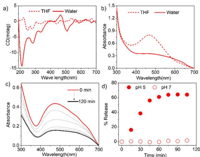
**Fig. 3** (a) CD and (b) UV/vis spectra of P1S in water and THF. (c) Time-dependent UV/vis spectra of P1S at pH 5 buffer solution. Each spectrum was taken at 15 min time intervals. (d) % release of NMIS from aqueous solution of P1S solution at pH 5 or pH 7 buffer (concentration of P1S = 1.0 mg mL<sup>-1</sup>).
