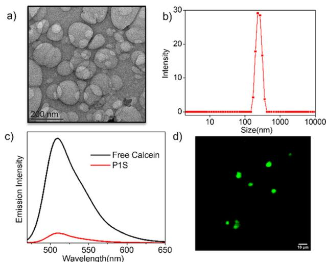
**Fig. 2** (a) TEM image ( $c = 0.1$  mg mL<sup>-1</sup>) and (b) DLS of P1S in water ( $c = 0.1$  mg mL<sup>-1</sup>). (c) Absorption normalized emission spectra ( $\lambda_{\text{ex}} = 450$  nm) of calcein encapsulated in P1S and free calcein in water. (d) Fluorescence microscopy image of the calcein-encapsulated P1S polymersome.
