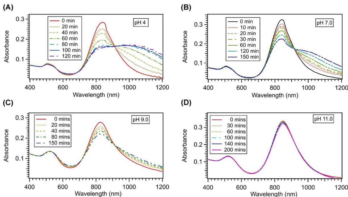
**Fig. 2** pH sensitivity of the end to end assembly of the Au NRs. Absorption spectra at different times after the addition of DTT monitoring the progress of the reaction at (A) pH 4.0, (B) pH 7.0, (C) pH 9.0, and (D) pH 11.0 respectively. With increasing pH the extent of the reaction decreases and at pH 11.0 the reaction completely stops.
