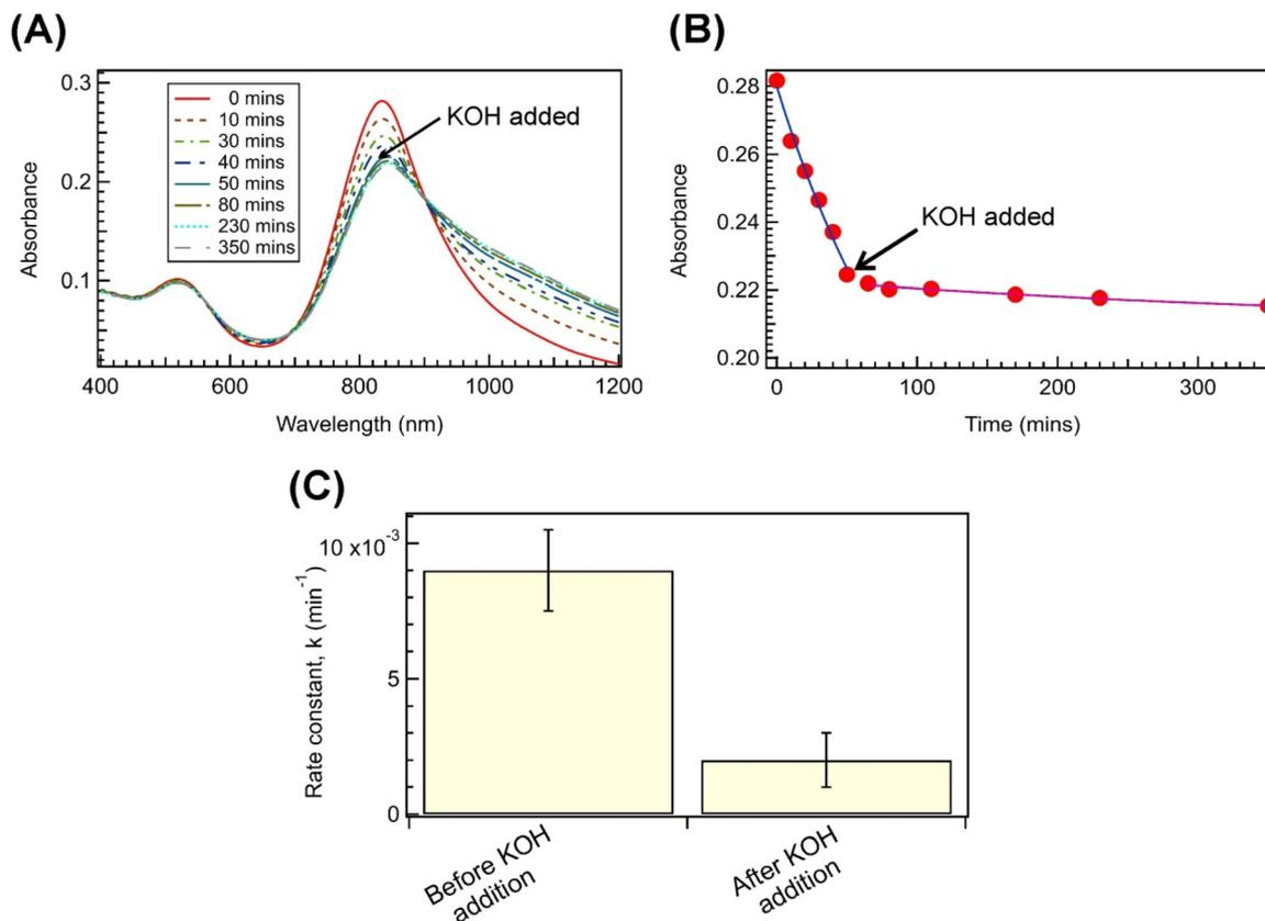
**Fig. 4** Results of the pH jump experiment. (A) Absorption spectra of the Au NRs at different times obtained in the pH jump experiment. At 50 minutes during the course of the reaction desired amount of KOH is added in the reaction medium to increase the pH from 4 to 11. (B) Plot of absorbance at  $\lambda_{\max}$  as a function of time. The time when KOH is added is shown by the arrow. (C) Bar plot showing the rate constant,  $k$  values before and after the addition of KOH.
