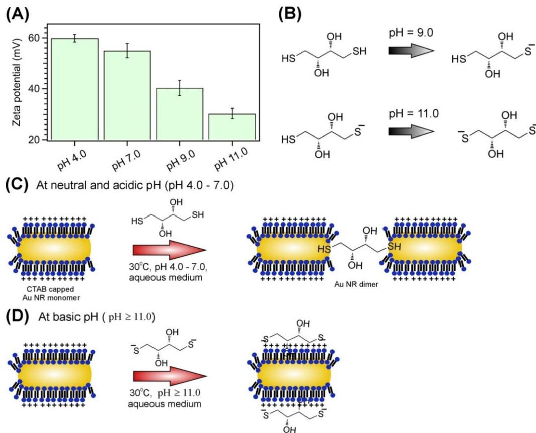
**Fig. 5** Mechanism of the pH controlled synthesis of end to end linked Au NR dimers. (A) Bar plot showing the zeta potential of Au NRs as a function of pH. (B) Schematics of the acid base chemistry of DTT at pH 9.0 and 11.0 respectively. (C) Graphical presentation of the end to end linking of Au NRs using DTT as a linker at neutral and acidic pH (pH 4.0 to 7.0). (D) Schematics of the reaction at pH  $\geq$  11.0.
