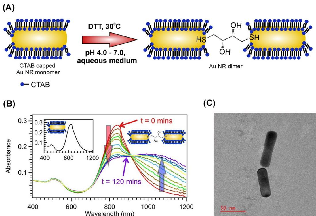
**Fig. 1** Preparation and characterization of Au NR dimer. (A) Schematic presentation of the Au NR dimer preparation from the Au NR monomer using the 1,4-dithiothreitol (DTT) as a linker in aqueous medium. (B) Absorption spectra as a function of time which monitor the progress of the dimer reaction over time in aqueous medium at pH 4.0. (C) Transmission electron microscopy (TEM) image of an Au NR dimer with a gap size  $\sim 1$  nm.
