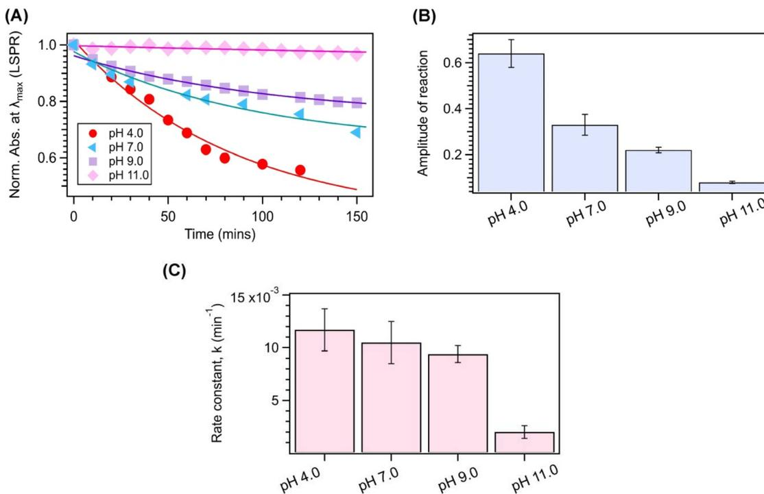
**Fig. 3** Amplitude and rate of the assembly reaction as a function of pH. (A) Plot of normalized absorbance at LSPR of the Au NRs as a function of time in aqueous solution for different pH. Here, symbols are the data and line is the monoexponential fit to the data. Plot of amplitude (B) and rate constant (C) of the assembly reaction as a function of pH.
