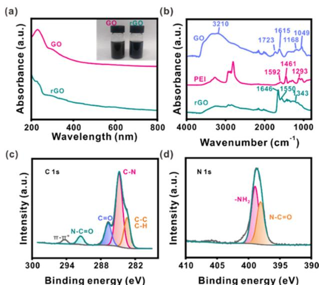
**Fig. 2** Characterization of GO and rGO. (a) UV-visible absorption spectra of rGO before and after modification. Inset: corresponding optical image of the samples. (b) Fourier-transform infrared spectra of GO, PEI, and rGO. XPS spectral analysis of rGO: (c) C 1s spectrum and (d) N 1s spectrum.
