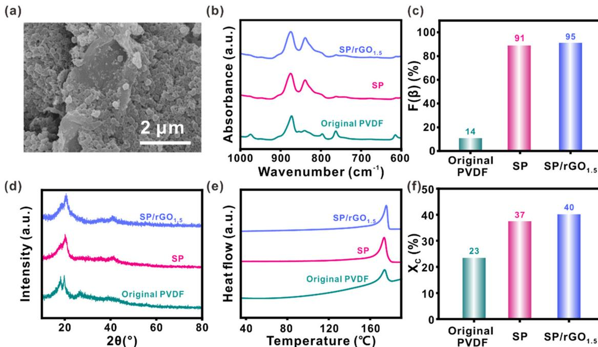
**Fig. 3** Characterization of self-polarized rGO/PVDF composites. (a) SEM image of the rGO/PVDF composite. (b) FTIR spectra of the PVDF starting material, self-polarized PVDF (SP), and self-polarized rGO/PVDF nanocomposites (SP/rGO<sub>x</sub>). (c) Corresponding calculated  $\beta$  phase content. (d) XRD pattern, (e) DSC heating curve, and (f) corresponding calculated crystallinity of various platforms.
