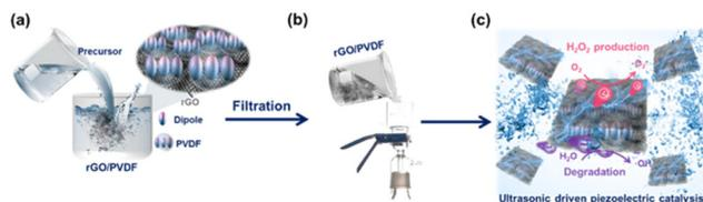
**Fig. 1** Schematic diagram of the preparation process of the self-polarized rGO/PVDF nanocomposite and its application in piezoelectric catalysis. (a and b) Preparation process of rGO/PVDF composites. (c) Application of rGO/PVDF in piezoelectric catalytic degradation of organic pollutants and  $\text{H}_2\text{O}_2$  production.
