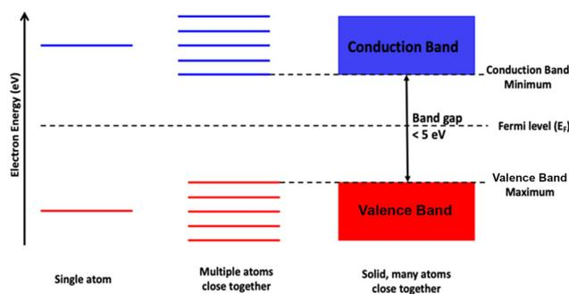
Fig. 3 Energy level and band diagram for semiconductors.
