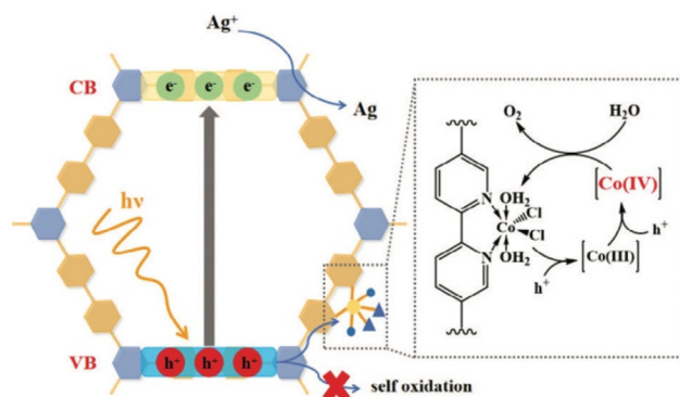
Fig. 17 Proposed mechanism for the photocatalytic water oxidation process facilitated by CoCl 2 -TpBPy. 324 Reproduced with permission from ref. 324. Copyright 2024, John Wiley and Sons.
