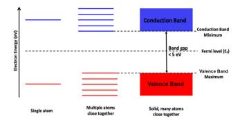
Energy level and band diagram for semiconductors.
