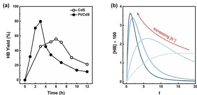
**Fig. 6** (a) HB yield of CdS and Pt/CdS NSs with Pt/Cd mass ratio of 0.017 during 12 h reaction. HB yield =  $2 \times n(\text{HB})/n_0(\text{BzOH}) \times 100\%$ ; (b) Relationship between [HB] and  $t$  in the eqn (11) at different appointed values of  $[\text{h}^+]$ . To enable the calculation by Python, we appointed the values of 0.24, 5, and 1 for  $[\text{BzOH}]_0$ ,  $k_1$ , and  $k_2$ , respectively. The initial value of [HB] is 0.
