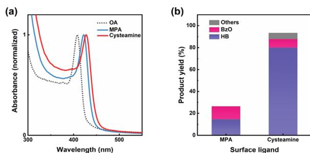
**Fig. 1** (a) Normalized absorption spectra of colloidal Pt/CdS NSs capped with OA in hexane, MPA in DMSO, and cysteamine in DMSO. (b) Products distribution of photocatalytic BzOH conversion by Pt/CdS NSs with different surface ligands. Yield (HB) =  $2 \times n(\text{HB})/n_0(\text{BzOH}) \times 100\%$ ; yield (BzO) =  $n(\text{BzO})/n_0(\text{BzOH}) \times 100\%$ ; yield (others) =  $100\% - \text{yield}(\text{HB}) - \text{yield}(\text{BzO})$ .
