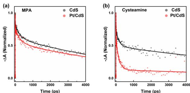
**Fig. 2** Normalized TA bleaching recovery kinetics of CdS NSs (grey) and Pt/CdS NSs (red): (a) at 422 nm with MPA as the capping ligand, and (b) at 424 nm with cysteamine as the capping ligand. The experimental data are represented by dots, with corresponding model fits from ESI Note 1† shown as solid lines.
