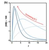
**Fig. 6** (a) HB yield of CdS and Pt/CdS NSs with Pt/Cd mass ratio of 0.017 during 12 h reaction. HB yield =  $2 \times n(\text{HB})/n_0(\text{BzOH}) \times 100\%$ ; (b) Relationship between [HB] and t in the eqn (11) at different appointed values of [h<sup>+</sup>]. To enable the calculation by Python, we appointed the values of 0.24, 5, and 1 for [BzOH]<sub>0</sub>,  $k_1$ , and  $k_2$ , respectively. The initial value of [HB] is 0.
