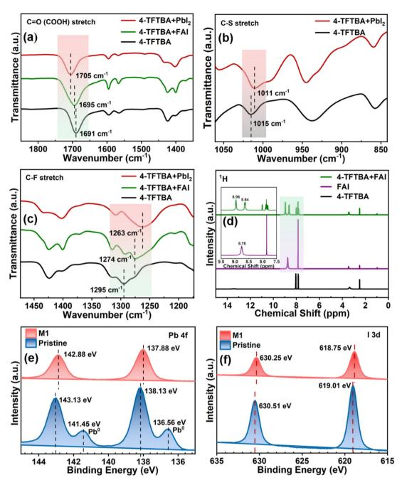
Fig. 2 FTIR spectra of (a) C=O, (b) C-S, and (c) C-F stretching vibration of 4-TFTBA with FAI and PbI<sub>2</sub> precursors; (d) <sup>1</sup>H NMR spectra of 4-TFTBA and 4-TFTBA + FAI; and XPS spectra of (e) Pb 4f and (f) I 3d orbital of the perovskite with and without modification by 4-TFTBA.
