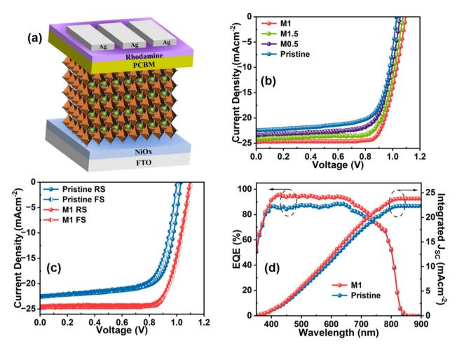
Fig. 5 (a) Schematic diagram of inverted PSC, (b) J-V curve of pristine and all modified devices, (c) J-V curve of the pristine and optimized devices in forward and reverse scan, (d) EQE spectra and integrated  $J_{SC}$  value of the pristine and optimized devices.
