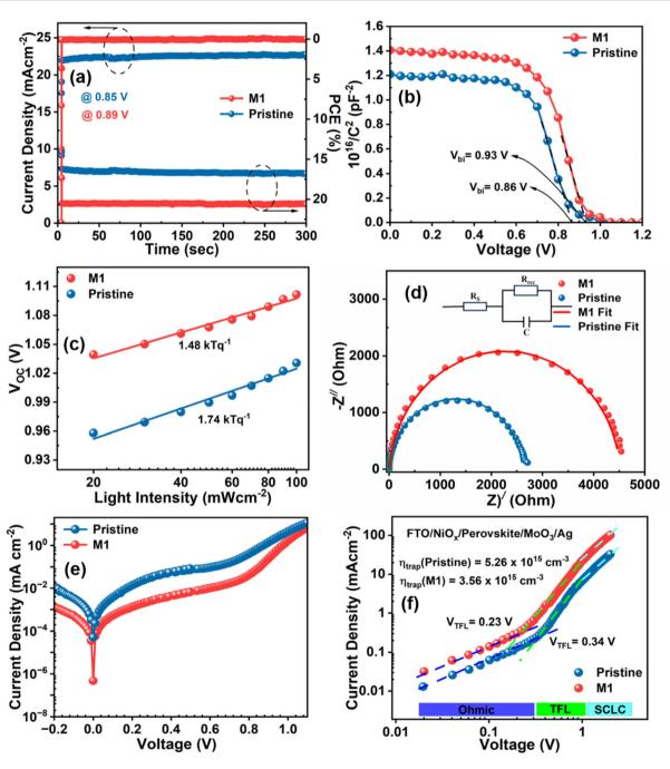
Fig. 6 (a) Stabilized photocurrent and PCE, (b) Mott-Schottky plot, (c) light intensity-dependent  $V_{\rm OC}$ , (d) Nyquist plot fitted with the respective equivalent circuit, (e) dark J-V plot, and (f) SCLC measurement of the hole-only-device of the pristine and optimized devices, respectively.
