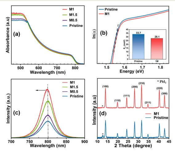
Fig. 3 (a) Absorption profile of pristine and all modified perovskite films, (b) Urbach energy calculation of pristine and optimized films, (c) steadystate photoluminescence spectra of pristine and all modified films, and (d) XRD of pristine and optimized perovskite films.
