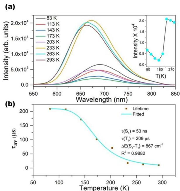
**Fig. 4** (a) Temperature-dependent emission spectra of  $\text{Ag}_{22}$  nanoclusters at 365 nm excitation. Inset: temperature-dependent solid-state photoluminescence intensity from 83 to 293 K. (b) Plot of photoluminescence lifetime at 670 nm against temperature for  $\text{Ag}_{22}$  and the data fitting. Reproduced from ref. 114 with permission from Wiley, copyright (2022).
