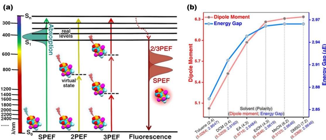
**Fig. 6** (a) Schematic illustration of single/two/three-photon excited fluorescence processes; (b) proportionality between solvent polarity and the simulated dipole moment/HOMO–LUMO energy gap of nanoclusters. Reproduced from ref. 131 with permission from Wiley, copyright (2022).
