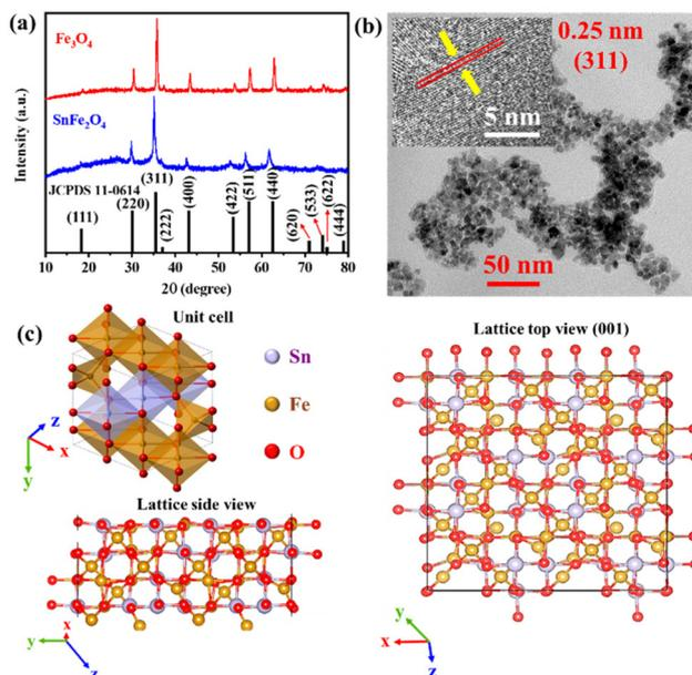
**Fig. 1** (a) PXRD pattern of as-synthesized SnFe<sub>2</sub>O<sub>4</sub> and Fe<sub>3</sub>O<sub>4</sub>. (b) HRTEM images of SnFe<sub>2</sub>O<sub>4</sub> along with atomic fringes for the exposed planes in the inset. (c) A polyhedral unit cell of the SnFe<sub>2</sub>O<sub>4</sub> lattice and the 2 × 2 supercell of the SnFe<sub>2</sub>O<sub>4</sub> layer showing top and side views of the lattice.
