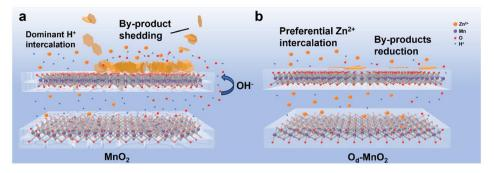
Fig. 1 The schematic diagram of the ion intercalation process of (a) MnO<sub>2</sub> and (b) O<sub>d</sub>-MnO<sub>2</sub>.
