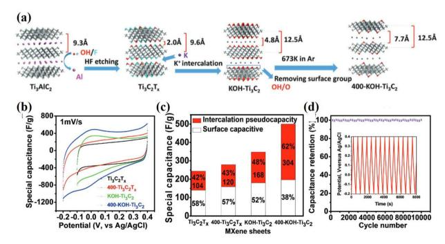
Fig. 14 (a) Synthesis scheme for modified MXene; (b) cycle voltammetry profiles at 1 mV s<sup>-1</sup> in 1 M H<sub>2</sub>SO<sub>4</sub>; (c) a comparative study of capacitance; (d) capacitance retention tests for the 400-KOH-Ti<sub>3</sub>C<sub>2</sub> electrode in 1 M H<sub>2</sub>SO<sub>4</sub>. Inset: galvanostatic cycling data collected at 1 A g<sup>-1</sup>. Reprinted with permission from ref. 246. Copyright 2017 John Wiley and Sons.
