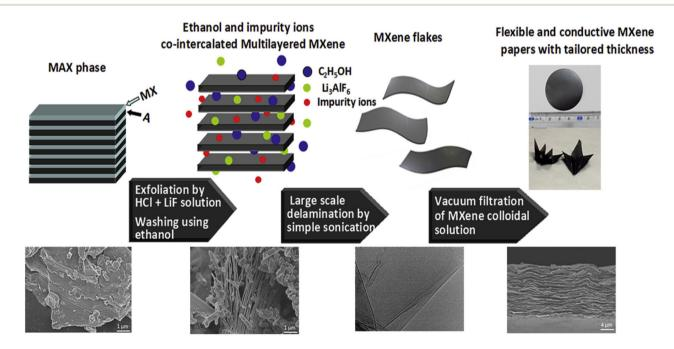
Fig. 2 MAX phase etching for the preparation of MXene through the HF/LiF method. Reprinted with permission from ref. 85. Copyright 2017
