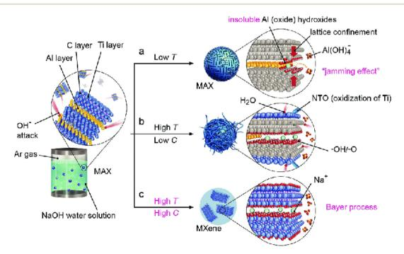
Fig. 4 A visual representation of the reaction between MAX and an aqueous solution of NaOH under different conditions: (a) at low temperature, (b) at high temperature and low NaOH concentration, and (c) at high temperature and high NaOH concentration. Reproduced with permission from ref. 98. Copyright 2018 John Wiley & Sons.
