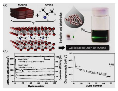
Fig. 12 (a) Schematic representation of the delamination process of  $Nb_2CT_x$  (MXene); (b) cycling stability and rate performance of  $Nb_2CT_x/CNT$  paper electrodes. Reprinted with permission from ref. 222. Copyright John Wiley and Sons.
