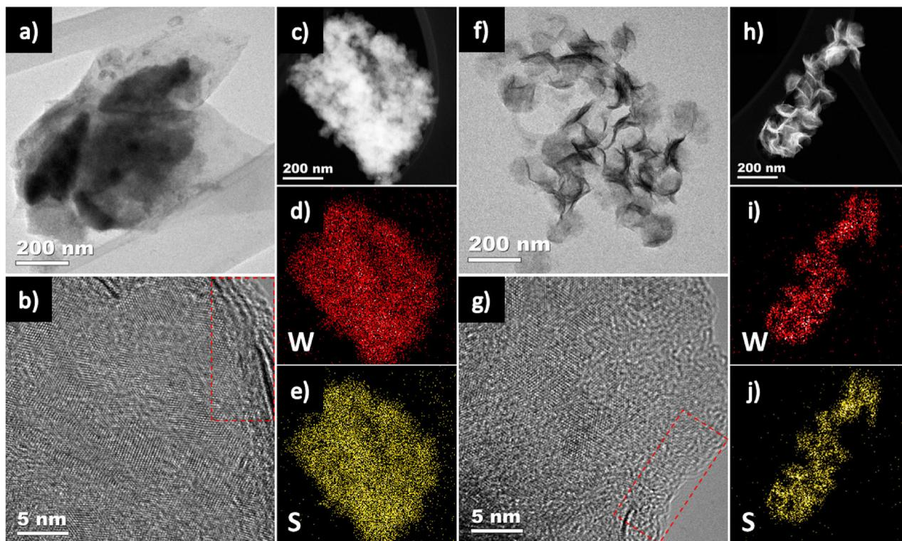
**Fig. 3** (a) TEM image, (b) HR-TEM image, and (c) STEM of NS-1T' with (d and e) corresponding elemental mapping for W and S. (f) TEM image, (g) HR-TEM image, and (h) STEM of NS-2H with (i and j) corresponding elemental mapping for W and S.
