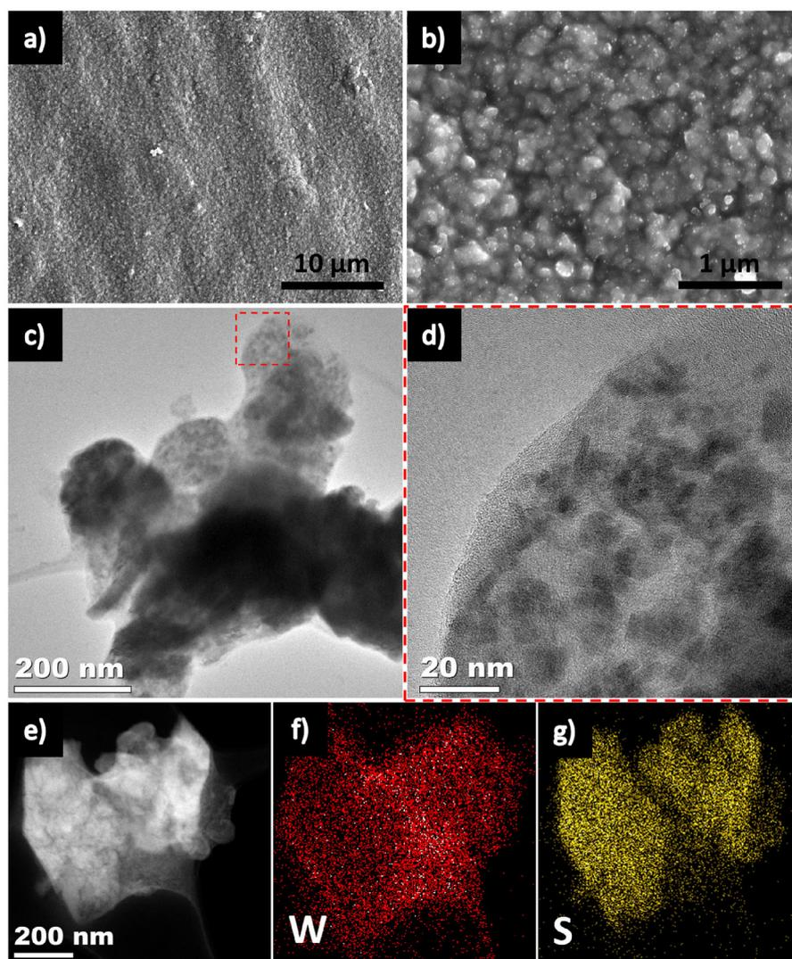
Fig. 6 Post-mortem after 100 cycles of WS<sub>2</sub> 2H: (a and b) SEM images, (c and d) TEM images, (e) STEM image and (f and g) elemental mapping of W and S of the NS-2H sample.
