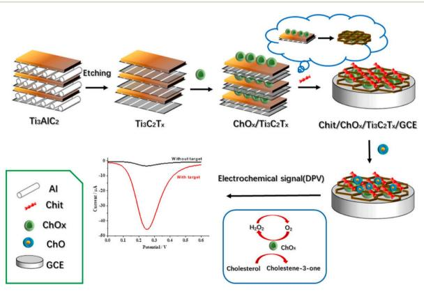
Fig. 10 The production method for  $Chit/ChO_x/Ti_3C_2T_x/GCE$  and the detection of cholesterol using the created biosensor. <sup>169</sup>
