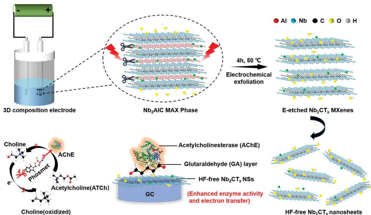
Fig. 11 The synthesis process for  $\text{Nb}_2\text{CT}_x$  MXene through an E-etching approach and the influence of the inhibition of enzymes on the ability of a biosensor based on  $\text{Nb}_2\text{CT}_x/\text{AChE}$  to identify phosmet.<sup>172</sup>
