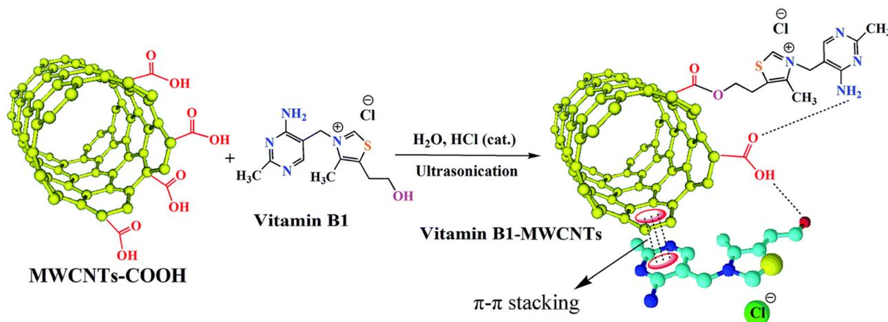
Fig. 3 The functionalization of MWCNTs with vitamin B1.<sup>97</sup>
