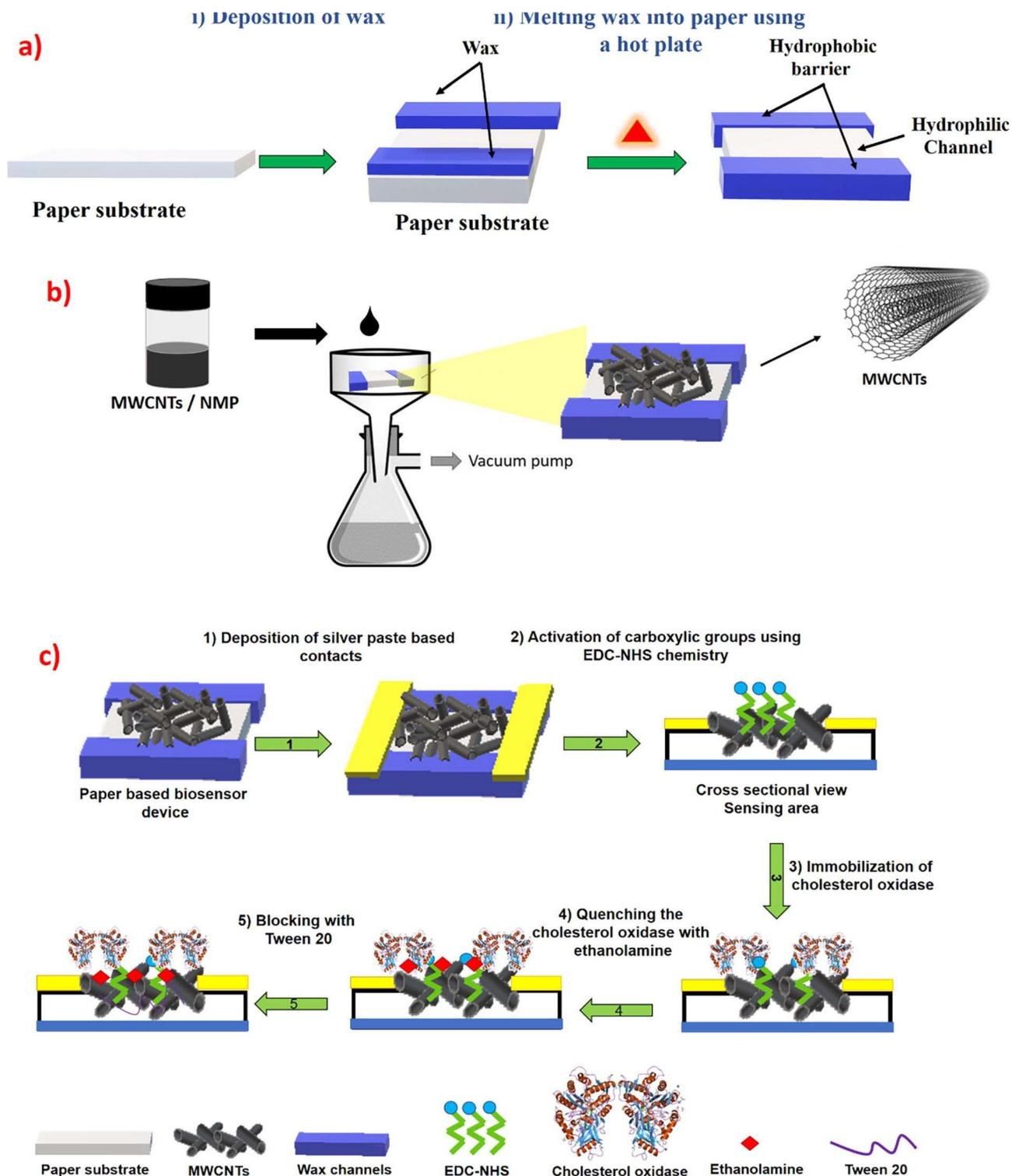
**Fig. 8** (a) Hydrophobic and hydrophilic pathways formed by the implantation of wax in the paper substrate. (b) MWCNTs are deposited on paper using a vacuum filtration process. (c) The covalent immobilization of  $\text{ChO}_x$  over the made-from-paper chemoresistive biosensor is demonstrated step by step.<sup>164</sup>
