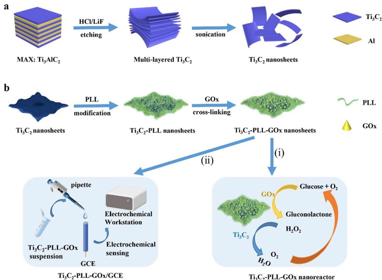
**Fig. 9** The synthesis procedure and glucose detection mechanism of the  $\text{Ti}_3\text{C}_2$ -PLL-GO<sub>x</sub> bio-sensor, (a) synthesizing process and (b) detection mechanism.<sup>168</sup>
