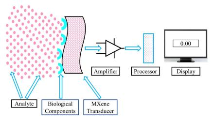
Fig. 1 Schematic working principle of biosensors.
