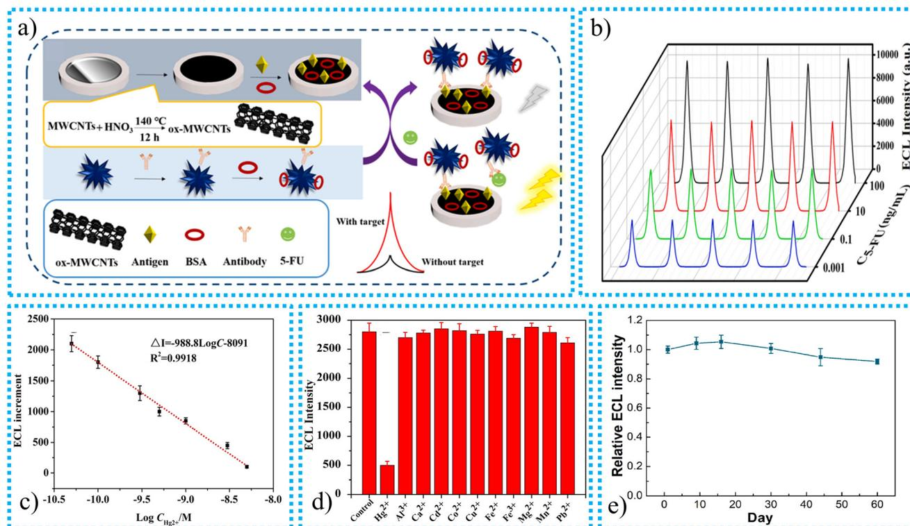
**Fig. 17** The synthesis mechanism for the CNT-based ECL sensor and the sensing mechanism for 5-FU, 5-cycle scan peaks of the immunosensor at various concentrations of analyte,<sup>185</sup> calibration graph of detection with ECL increments, (c) selectivity analysis,<sup>194</sup> (d) stability of the SEES using the Ru/CNT/graphene electrode over two months of storage.<sup>187</sup>
