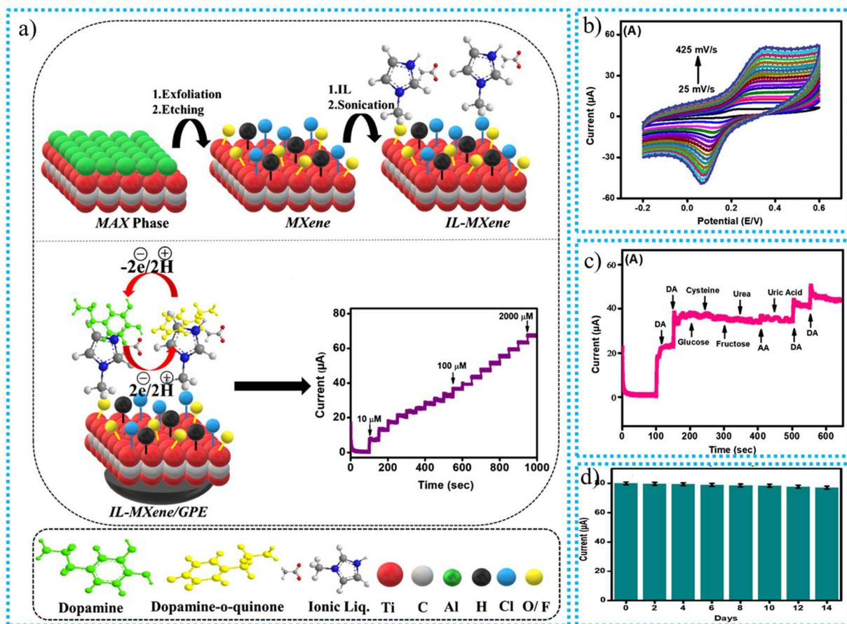
Fig. 18 The MXene-based ECL sensor: (a) synthesis procedure and the sensing mechanism to detect DA, (b) CV response, (c)  $40 \mu M$  DA (first 2 spikes),  $20 \mu M$  DA (last 2 spikes), and  $500 \mu M$  interfering molecules, (d) stability.<sup>190</sup>
