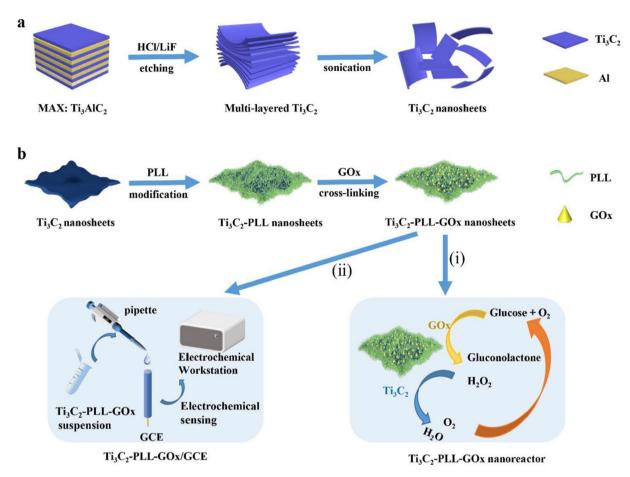
Fig. 9 The synthesis procedure and glucose detection mechanism of the  $Ti_3C_2$ -PLL-GO<sub>x</sub> bio-sensor, (a) synthesizing process and (b) detection mechanism.168
