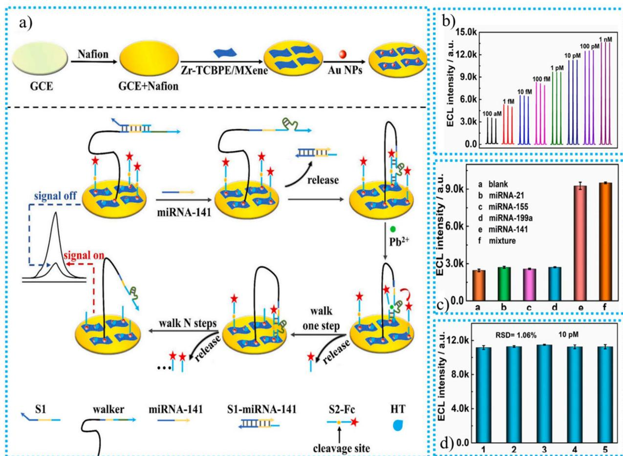
**Fig. 19** (a) The hairpin-free and nuclease-free amplification methods with DNAzyme assistance and MXene-based Zr-TCBPE/MXene ECL sensor, (b) ECL responses of the sensing platform toward several concentrations of miRNA-141 (100 aM–1 nM), MXene-based Zr-TCBPE/MXene ECL, (c) selectivity, (d) reproducibility.<sup>192</sup>
