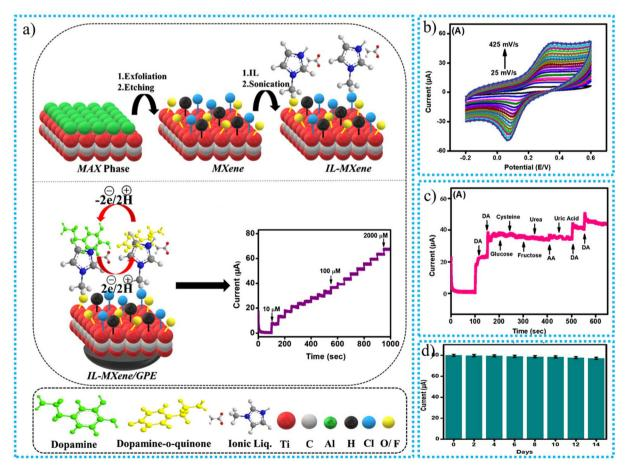
Fig. 18 The MXene-based ECL sensor: (a) synthesis procedure and the sensing mechanism to detect DA, (b) CV response, (c) 40 µM DA (first 2 spikes), 20 µM DA (last 2 spikes), and 500 µM interfering molecules, (d) stability. 190
