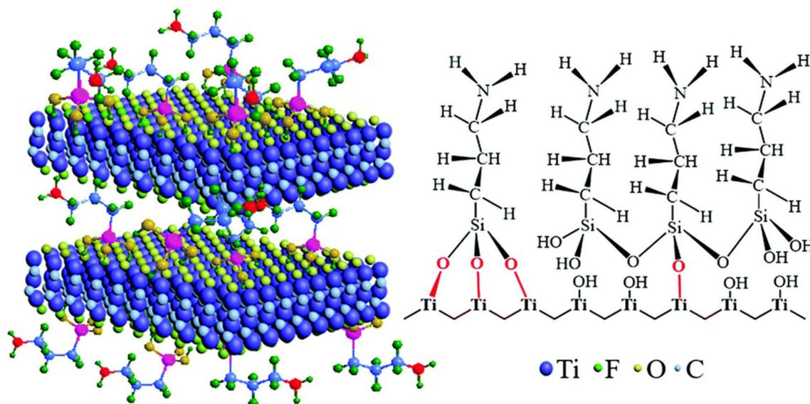
Fig. 4 The alkalization–grafting procedure for producing Ti<sub>3</sub>C<sub>2</sub>T<sub>x</sub> MXene nanosheets with amino functionalities.<sup>108</sup>
