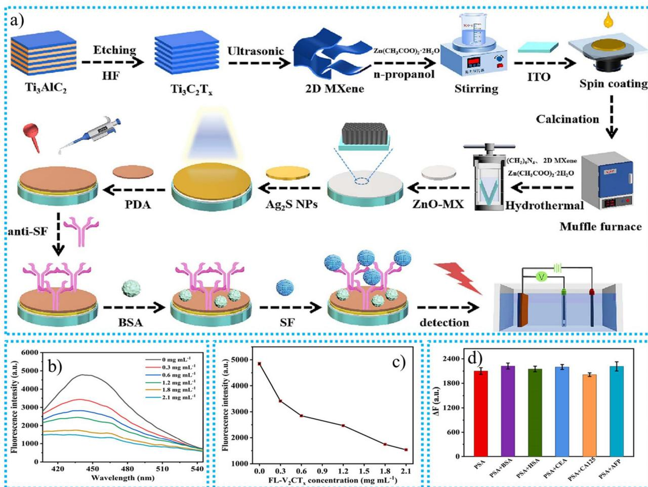
Fig. 16 (a) The ZnO-MX/Ag<sub>2</sub>S nanomaterial development procedure and the PEC immunosensor development procedure,<sup>180</sup> (b) fluorescence emission spectra, (c) fluorescence intensity of aptamer-CGQDs with FL-V<sub>2</sub>CT<sub>x</sub> concentrations, (d) ΔF of the aptasensor for PSA in the presence of 3-fold BSA, HSA, CEA, CA125, and AFP, respectively. Conditions: PSA concentration was 15 ng mL<sup>-1</sup>.<sup>182</sup>
