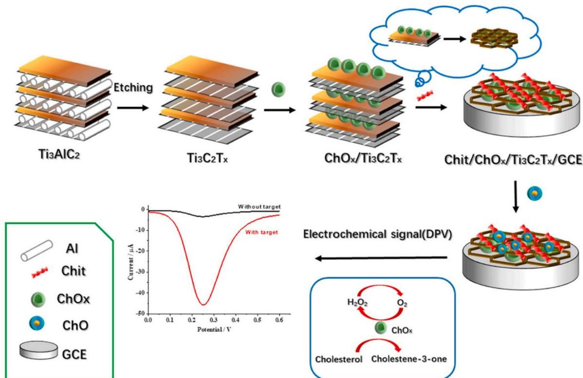
Fig. 10 The production method for Chit/ $\text{ChO}_x$ / $\text{Ti}_3\text{C}_2\text{T}_x$ /GCE and the detection of cholesterol using the created biosensor.<sup>169</sup>
