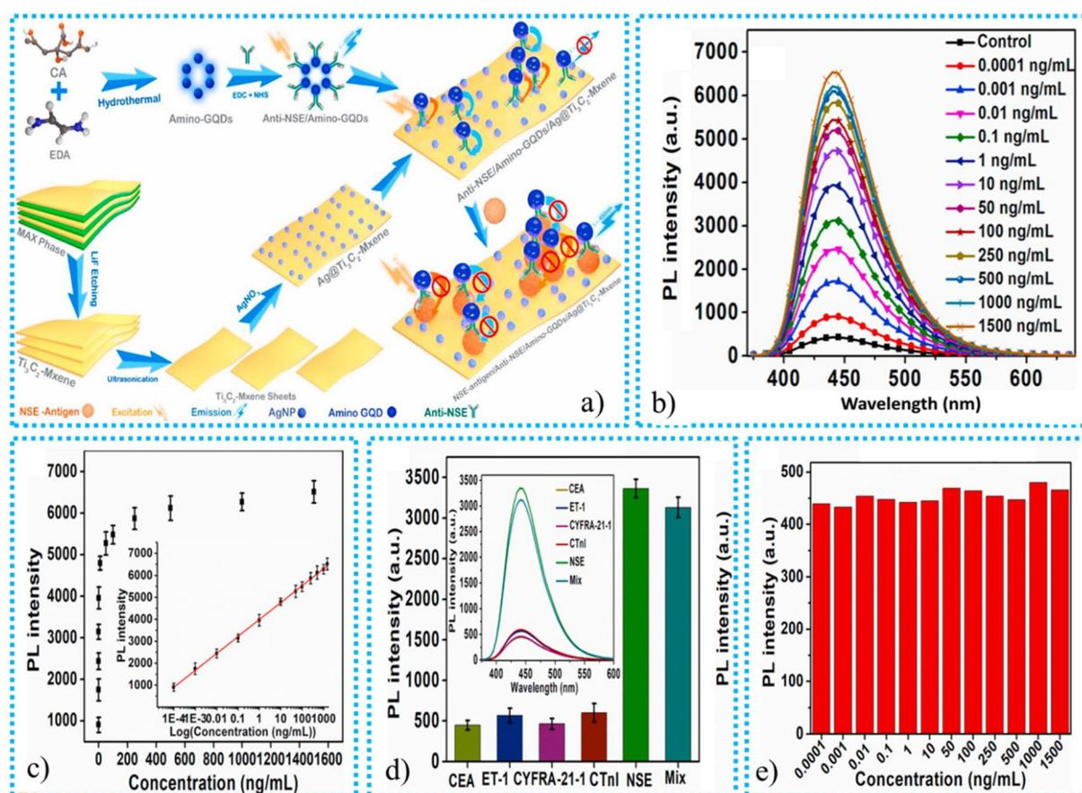
**Fig. 15** (a) The NSE sensing mechanism for the MXene-based immunosensor, (b) analytical performance of the MXene-based fluorescent biosensor, (c) the graph of recovered fluorescence vs. different NSE concentrations, in the range of  $0.0001\text{--}1500 \text{ ng mL}^{-1}$ , (d) selectivity of the biosensors, (e) control experiment for the amino-GQDs/ $\text{Ag}@\text{Ti}_3\text{C}_2\text{-MXene}$  immunoelectrode.<sup>179</sup>
