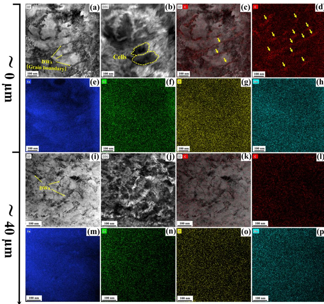
**Fig. 7** (a) Bright-field image, (b) DF4-STEM image and (c)–(h) EDS elemental mapping of the USPed sample with the peening duration of 8 min at its topmost surface indicating carbon segregation at grain boundaries; (i) bright-field image, (j) HAADF-STEM image; and (k)–(p) EDS elemental mapping of the USPed sample with the peening duration of 8 min at the location of 40 μm depth from its topmost surface.
