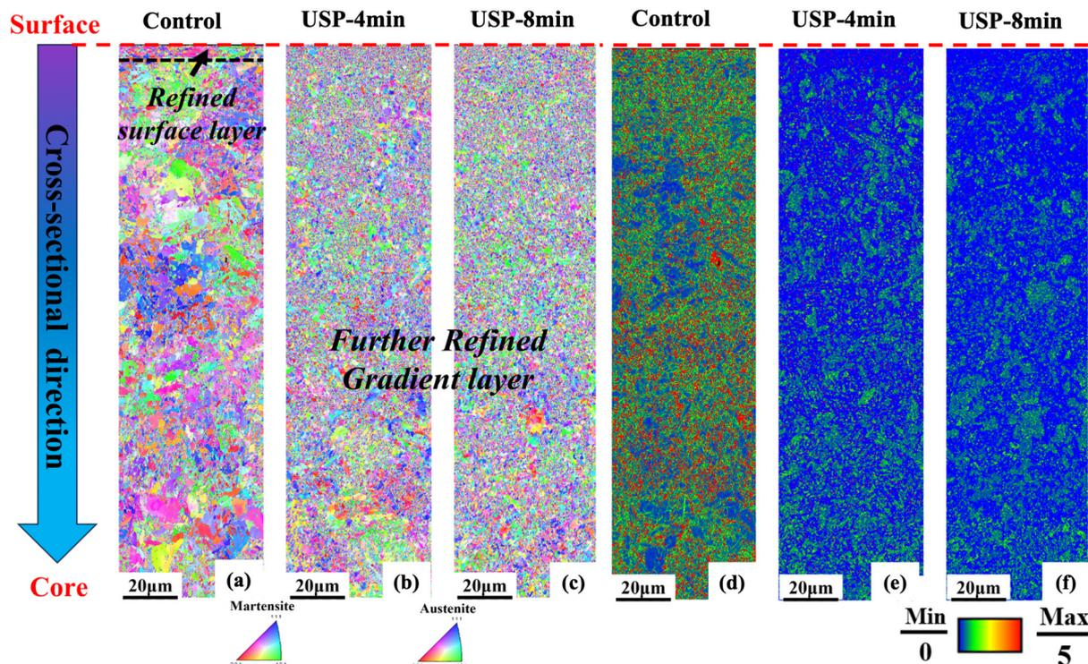
**Fig. 14** Inverse pole figure (IPF) characterization of the bearing steel sample after wear tests: (a) the coarse-grained GCr15 bearing steel sample (control) and the USPed GCr15 bearing steel sample with peening durations of (b) 4 min (USP-4 min) and (c) 8 min (USP-8 min) and kernel average misorientation (KAM) mapping of the (d) control sample, (e) the USP-4 min sample and (f) the USP-8 min sample after the sliding wear tests.
