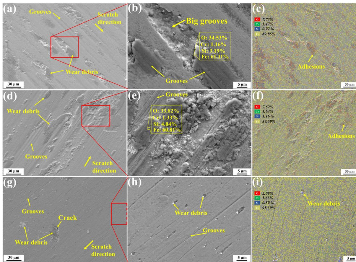
**Fig. 13** SEM characterization of the worn surface of the (a) as-received and USPed GCr15 bearing steel sample with peening durations of (d) 4 min and (g) 8 min; (b), (e) and (h) magnified observations of the areas indicated by the red rectangles in (a), (d) and (g), respectively; and (c), (f) and (i) EDS mapping of the worn surface of the as-received and USPed GCr15 bearing steel sample with peening durations of 4 min and 8 min, respectively.
