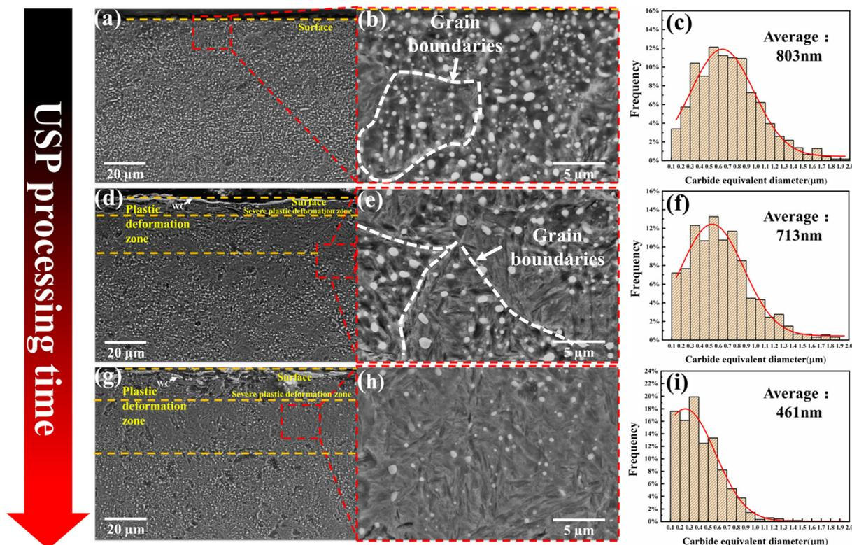
**Fig. 2** SEM images of (a) and (b) the as-received GCr15 bearing steel, (d) and (e) the USPed GCr15 bearing steel with the peening duration of 4 min, and (g) and (h) USPed GCr15 bearing steel with the peening duration of 8 min, along the cross-sectional direction. (c), (f) and (i) Statistical analysis of the size of the carbides in the sample with respect to peening durations of 0 min, 4 min and 8 min. The white dashed lines indicate grain boundaries.
