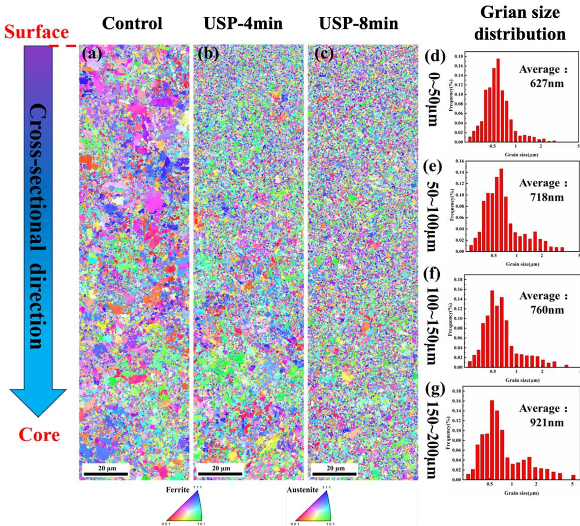
**Fig. 3** Inverse pole figure (IPF) EBSD mapping of the (a) as-received control sample and the USPed sample with peening durations of (b) 4 min and (c) 8 min along the cross-sectional direction. (d)–(g) Statistical analysis of the phase size in the gradient nanostructured GCr15 bearing steel with the peening duration of 8 min along its cross-sectional direction.
