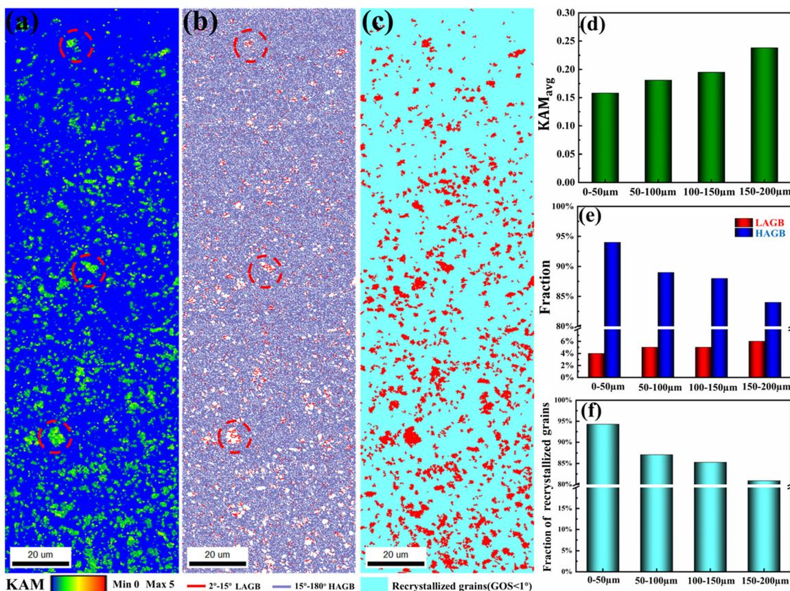
**Fig. 12** (a) KAM, (b) grain boundary and (c) GOS mapping of the gradient nanostructured GCr15 bearing steel fabricated by USP with the peening duration of 8 min; statistical analysis of the (d) average value of KAM; (e) fractions of grain boundaries; and (f) fractions of the recrystallized grains of the gradient nanostructured GCr15 bearing steel at different depths.
