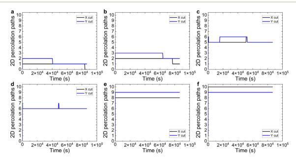
Fig. 8 Number of two-dimensional percolation paths within the CF structure for the 6 distinct LRSs employed in our study: (a) LRS1, (b) LRS2, (c) LRS3, (d) LRS4, (e) LRS5, and (f) LRS6.
