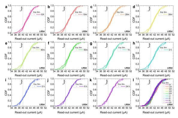
Fig. 5 Comparative representation of the read-out current CDFs, corresponding to LRS4, obtained from experimental (dots) and simulated (lines) data for a sample set comprising 128 distinct devices. Eleven time steps were considered: (a) EA (0 min), (b) 10 min, (c) 20 min, (d) 30 min, (e) 40 min, (f) 50 min, (g) 1 h, (h) 2 h, (i) 5 h, (j) 8 h, (k) 24 h, (l) all the data plotted together.
