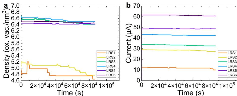
**Fig. 10** (a) Comparison of CF density for a particular device over time, for the 6 different conductance levels under consideration, (b) simulated read-out current of one particular device as a function of time for the multilevel operation under study: LRS1, LRS2, LRS3, LRS4, LRS5, and LRS6.
