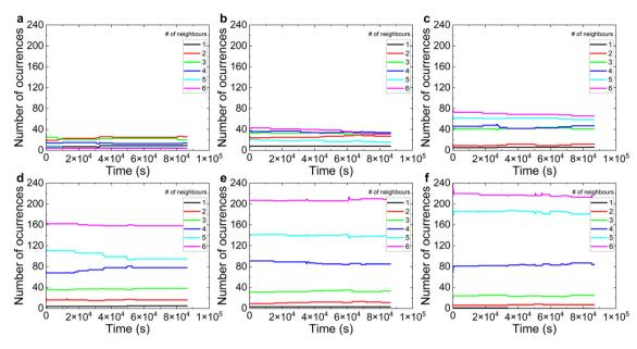
Fig. 9 Time evolution of the number of oxygen vacancies with a determined number of neighbors in the CF for the 6 different conductance levels under consideration: (a) LRS1, (b) LRS2, (c) LRS3, (d) LRS4, (e) LRS5, and (f) LRS6.
