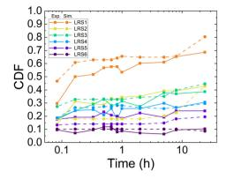
Fig. 7 CDF of the failure rate as a function of the time observed in a sample of 128 individual devices, categorized into 6 distinct low resistance states (LRS1–LRS6) for the experimental data (squares) and simulations (circles).
