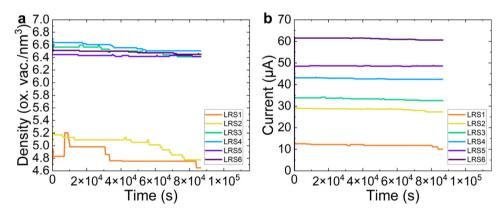
Fig. 10 (a) Comparison of CF density for a particular device over time, for the 6 different conductance levels under consideration, (b) simulated read-out current of one particular device as a function of time for the multilevel operation under study: LRS1, LRS2, LRS3, LRS4, LRS5, and LRS6.
