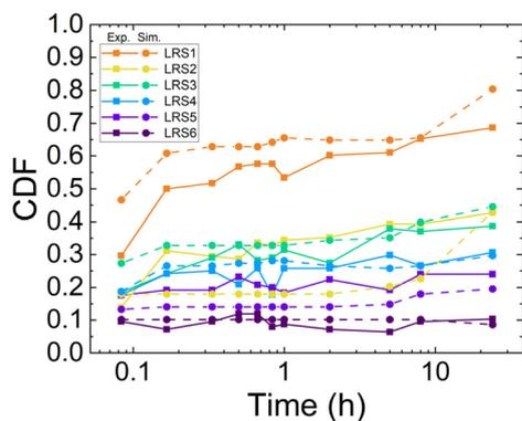
**Fig. 7** CDF of the failure rate as a function of the time observed in a sample of 128 individual devices, categorized into 6 distinct low resistance states (LRS1–LRS6) for the experimental data (squares) and simulations (circles).
