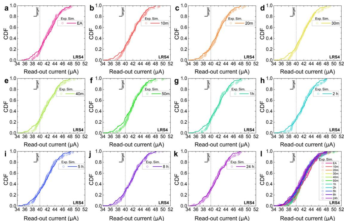
**Fig. 5** Comparative representation of the read-out current CDFs, corresponding to LRS4, obtained from experimental (dots) and simulated (lines) data for a sample set comprising 128 distinct devices. Eleven time steps were considered: (a) EA (0 min), (b) 10 min, (c) 20 min, (d) 30 min, (e) 40 min, (f) 50 min, (g) 1 h, (h) 2 h, (i) 5 h, (j) 8 h, (k) 24 h, (l) all the data plotted together.
