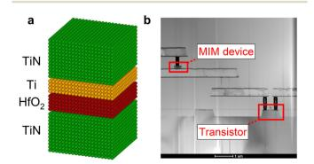
Fig. 1 (a) Layer MIM stack scheme of the devices measured, (b) crosssection TEM image of the 1T1R structure tested within the crossbar
