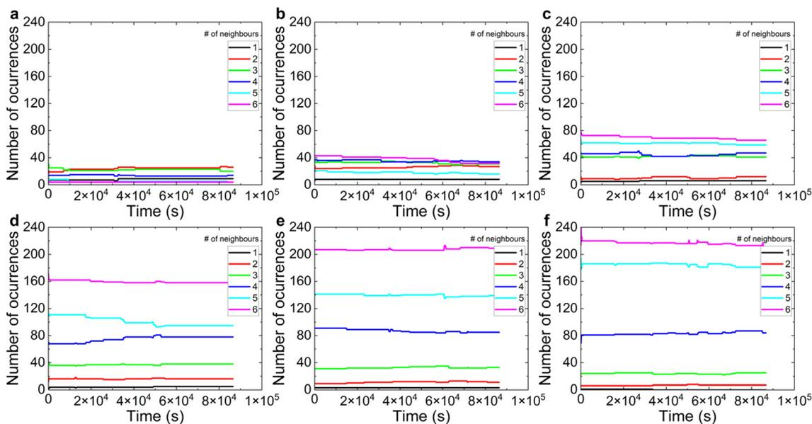
**Fig. 9** Time evolution of the number of oxygen vacancies with a determined number of neighbors in the CF for the 6 different conductance levels under consideration: (a) LRS1, (b) LRS2, (c) LRS3, (d) LRS4, (e) LRS5, and (f) LRS6.
