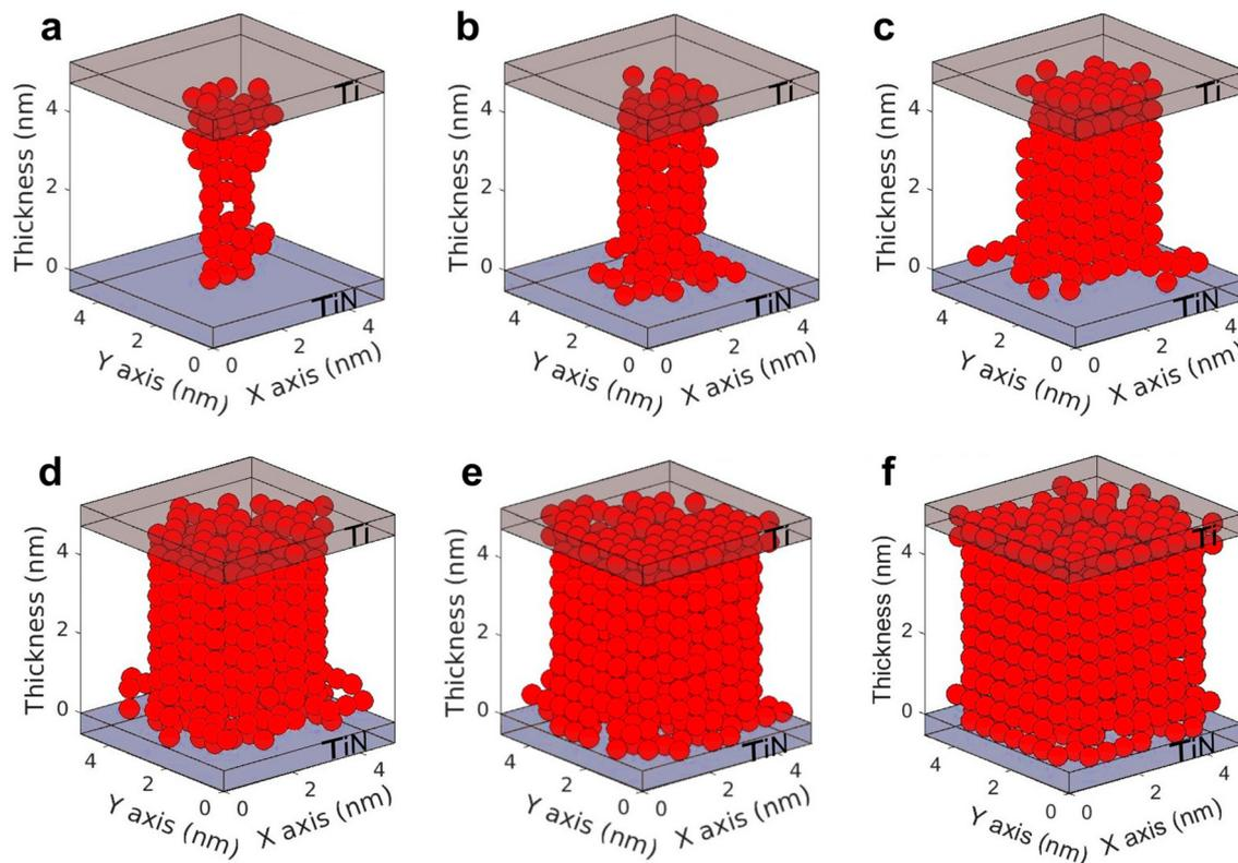
**Fig. 3** Plot of the oxygen vacancies in the simulation domain (corresponding to the dielectric) of fully-formed CFs in simulated devices with a conductance that corresponds to the 6 distinct experimental LRS obtained with ISPVA: (a) LRS1, (b) LRS2, (c) LRS3, (d) LRS4, (e) LRS5, (f) LRS6.
