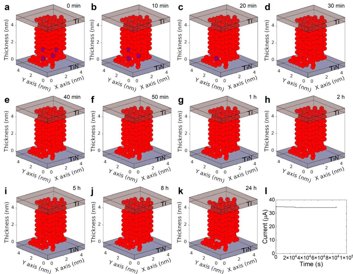
**Fig. 4** (a–k) KMC simulated CF evolution for a device in the LRS3. Prior to the test, an initialization simulation is performed to create a CF. As can be seen in the simulated experiment, a very slight morphological CF degradation is produced over time. Red balls depict oxygen vacancies and purple ones denote grid points where both an oxygen vacancy and an oxygen ion (not recombined) are present. (l) Read-out current versus time obtained during the simulation.
