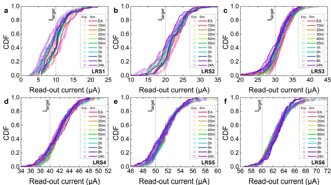
**Fig. 6** Comparative representation of the read-out current CDFs obtained from experimental (dots) and simulated (lines) data in a sample set comprising 128 distinct devices, covering eleven time steps: EA (0 min), 10 min, 20 min, 30 min, 40 min, 50 min, 1 h, 2 h, 5 h, 8 h, and 24 h. The analysis encompasses 6 distinct LRS: (a) LRS1, (b) LRS2, (c) LRS3, (d) LRS4, (e) LRS5, (f) LRS6.
