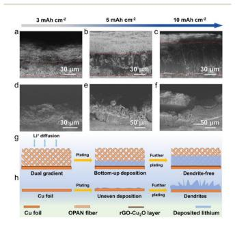
Fig. 2 Side-view SEM images of Li deposition in (a-c) OGCC and (d-f) bare Cu foil at 0.5 mA cm<sup>-2</sup>: (a and d) 3 mA h cm<sup>-2</sup>; (b and e) 5 mA h cm<sup>-2</sup>; and (c and f) 10 mA h cm<sup>-2</sup>. Schematic illustrations of Li deposition in (g) OGCC and (h) bare Cu foil.
