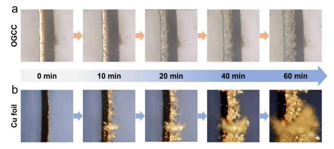
Fig. 3 In situ optical images of the Li plating process in (a) OGCC and (b) bare Cu foil.
