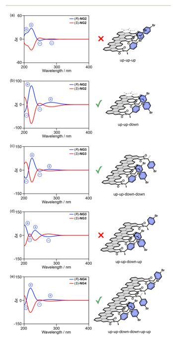
Fig. 18 (a)-(e) Calculated CD spectra of model edge structures with (a) up-up-up, (b) up-up-down, (c) up-up-down-down, (d) up-updown-up, and (e) up-up-down-down-up-up orientations (ref. 71). Copyright 2024 Wiley-VCH.
