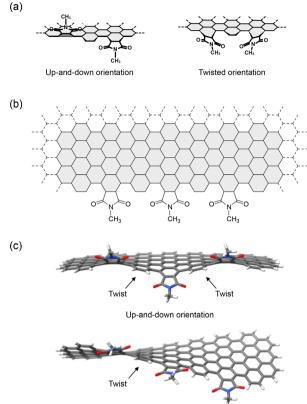
Fig. 12 (a) Up-and-down (left) and twisted orientations (right). (b) Chemical structure of the model edge used for the DFT calculations. (c) Optimized structures of the model edge carrying N-methyl five-membered imides on the edge. Color scheme: gray (carbon), white (hydrogen), blue (nitrogen), red (oxygen) (ref. 5). Copyright 2023, Wiley-VCH.
