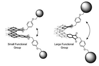
Fig. 16 Schematic representation of (left) small and (right) large substituents on the edge. The latter may cause a larger twist on the edge (ref. 12). Copyright 2016, Wiley-VCH.
