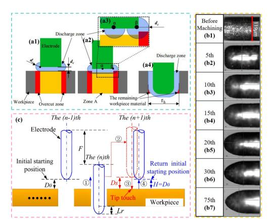
Fig. 5 (a1–a4) Schematic diagram of the electrode wear process: (a1) discharge start; (a2) electrode feed; (a3) partial enlarged view of the discharge gap; (a4) perforation formation.<sup>57</sup> (b1–b7) Evolution of electrode morphology during the array micro-hole machining process.<sup>57</sup> (c) Schematic diagram of the compensation strategy for online contact measurement.<sup>59</sup>
