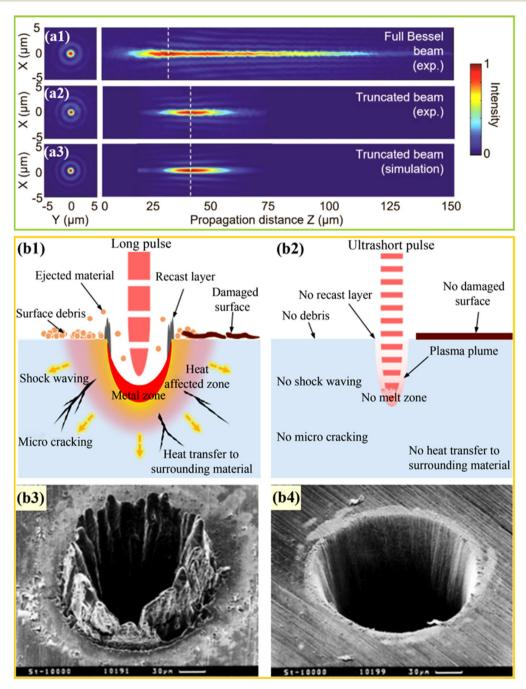
Fig. 7 (a1-a3) Distribution of Bessel beam intensity on the surface of fused silica: (a1) Bessel beam; (a2) experimental truncated Bessel beam; (a3) simulated truncated Bessel beams.<sup>87</sup> (b1-b4) Comparison of ultrafast laser and long pulse laser drilling: (b1) schematic diagram of long pulse laser drilling; (b2) schematic diagram of ultrafast laser drilling; (b3) SEM images of holes processed by a long pulse laser; (b4) SEM images of holes processed by an ultrafast laser.88
