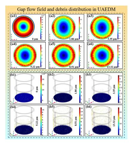
Fig. 18 (a) Distribution of the gap flow field under different ultrasonic amplitudes: (a1) 0 μm; (a2) 1.86 μm; (a3) 3.35 μm; (a4) 5.22 μm; (a5) 8.51 μm; (a6) 13.32 μm. (b) Debris removal under two vibration cycles corresponding to different ultrasonic amplitudes: (b1) 0 μm; (b2) 1.86 μm; (b3) 3.35 μm; (b4) 5.22 μm; (b5) 8.51 μm; (b6) 13.32 μm.  $^{196}$
