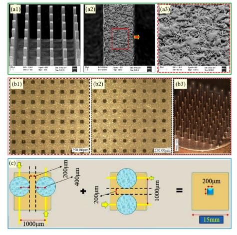
Fig. 4 (a1–a3) Array electrodes prepared by low-speed wire EDM: (a1) panorama; (a2) enlarged view; (a3) local morphology map.<sup>52</sup> (b1–b3) Cylindrical array electrodes prepared by self-loss precision machining: (b1) array micro-hole inlet; (b2) array micro-hole outlet; (b3) picture of array electrodes.<sup>53</sup> (c) Schematic diagram of the array electrode machining strategy.<sup>54</sup>
