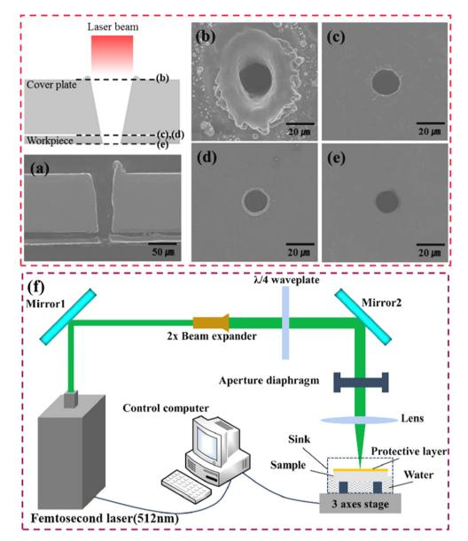
Fig. 8 Laser processed hole on the cover plate. (a) Overall morphology of holes; (b-e) hole morphology diagram at the corresponding crosssection;<sup>101</sup> (f) schematic diagram of a laser processing device assisted by a protective layer and a water layer.<sup>102</sup>
