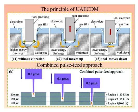
Fig. 20 (a) The effect of ultrasonic vibration on spark energy distribution: (a1) no ultrasonic vibration; (a2) upward movement of tools; (a3) downward movement of tools;<sup>217</sup> (b) schematic diagram of the combined pulse feed method.<sup>220</sup>
