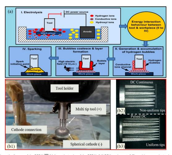
Fig. 19 (a) Schematic diagram of the ECDM.<sup>200</sup> (b) Array electrodes of the ECDM: (b1) ECM equipment; (b2) repairing array electrodes with a pulse power supply; (b3) the restored array electrodes repaired with a continuous power supply.<sup>206</sup>
