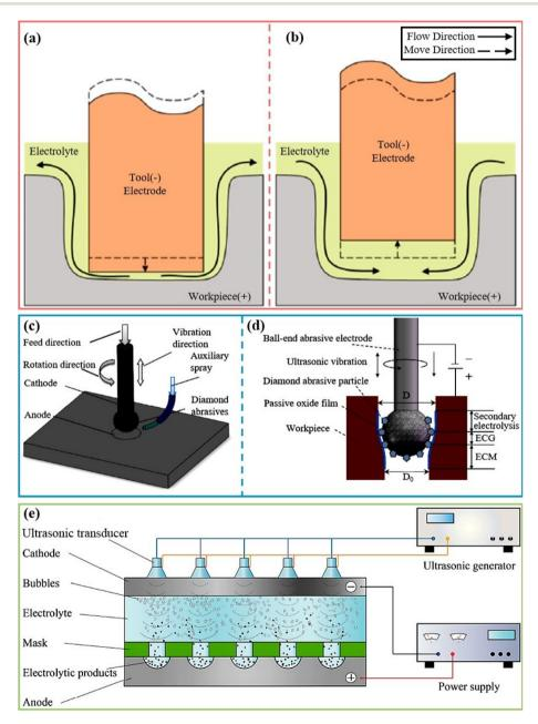
Fig. 17 (a and b) Schematic diagram of the ultrasonic pumping effect: (a) tool electrode moving downward; (b) tool electrode moving upward.<sup>39</sup> (c and d) Schematic diagram of the UAECDG machining principle: (c) schematic diagram of the processing area; (d) UAECDG processing mechanism diagram. <sup>184</sup> (e) Schematic diagram of the ultrasonic assisted mask electrochemical machining principle. <sup>185</sup>
