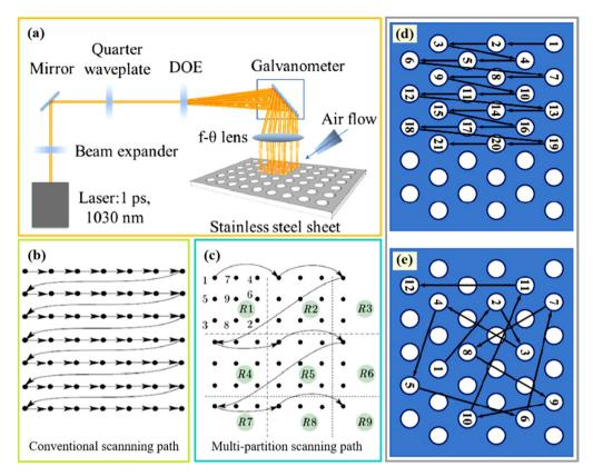
Fig. 9 (a) Schematic diagram of the multi-beam laser processing principle; (b) schematic diagram of the traditional scanning path; (c) schematic diagram of the heat input regulation path strategy. (d) Linear scanning strategy; (e) random scanning strategy. 114
