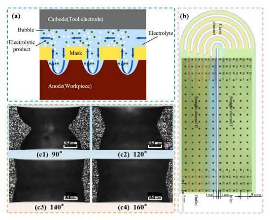
Fig. 14 (a) Schematic diagram of the processing principle of TMEMM. (b) Schematic diagram of the optimized serpentine flow channel. (c) Cross section of holes under different mask wall angles: (c1) 90°; (c2) 120°; (c3) 140°; (c4) 160°.
