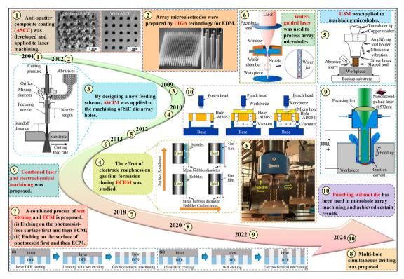
Fig. 2 Development of important processes for array micro-hole machining. 14,22,25–32
