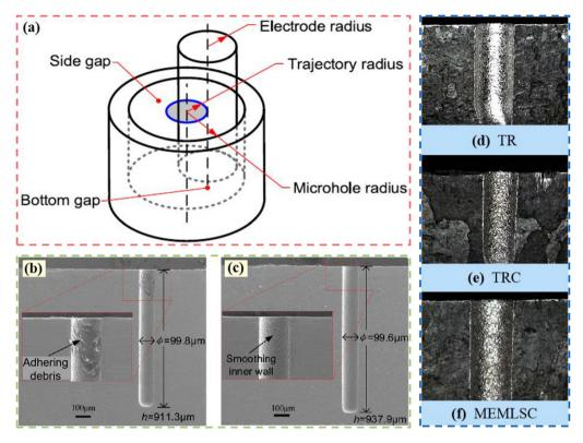
Fig. 6 (a) Schematic diagram of the UCV electrode machining principle. (b) SEM pictures of micro-holes processed by rotating electrodes. (c) SEM pictures of micro-holes processed by UCV electrodes. (d–f) Profile diagram of micro-holes processed by different pulse generators: (d) TR pulsed generator; (e) TRC pulsed generator; (f) MEMLSC pulsed generator.
