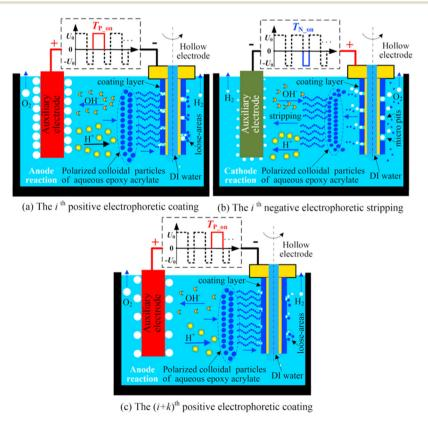
Fig. 12 Asymmetric timed bipolar electrophoresis coating process: (a) the i<sup>th</sup> positive electrophoretic coating; (b) the i<sup>th</sup> negative electrophoretic stripping; (c) the  $(i + k)^{th}$  positive electrophoretic coating.<sup>130</sup>
