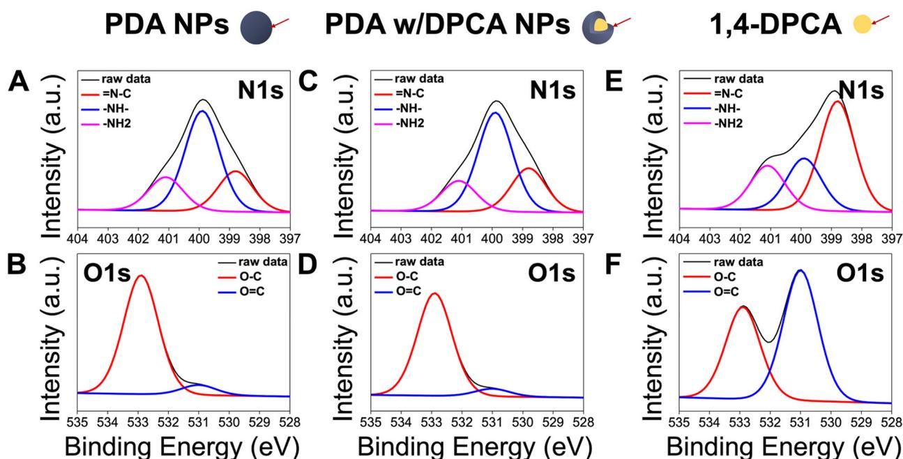
**Fig. 3** High-resolution N1s and O1s XPS spectra of (A and B) PDA NPs, (C and D) PDA NPs with DPCA, and (E and F) 1,4-DPCA.
