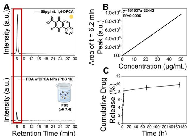
**Fig. 4** (A) Confirmation of drug release from PDA w/DPCA NPs, (B) standard curve for the calculation of drug release using various concentrations of 1,4-DPCA. (C) *In vitro* drug release profile of PDA w/DPCA NPs. a.u. denotes arbitrary unit.
