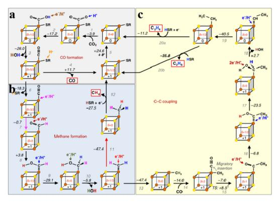
Fig. 5 Mechanism of CO<sub>2</sub> reduction catalyzed by Fe-S clusters. (a) Fe-S clusters catalyze CO formation. (b) Fe-S clusters catalyze methane formation. (c) Fe-S clusters catalyze C-C coupling. Reproduced with permission from ref. 26. Copyright 2018, Springer Nature.
