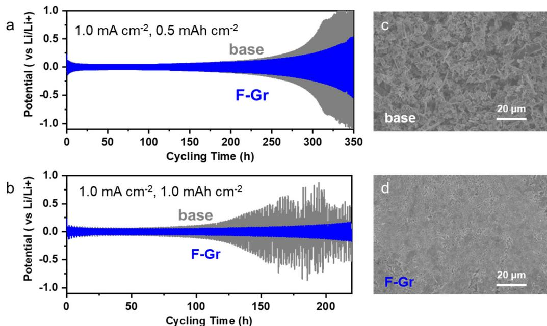
**Fig. 1** Electrochemical performance of Li/Li symmetrical cell with the plating capacity of (a)  $0.5 \text{ mA h cm}^{-2}$  and (b)  $1.0 \text{ mA h cm}^{-2}$ , respectively (base: gray trace; F-Gr: blue trace). SEM images of the Li-metal surface in the electrolyte (c) without and (d) with F-Gr after 50 cycles at the current density of  $1 \text{ mA cm}^{-2}$ .
