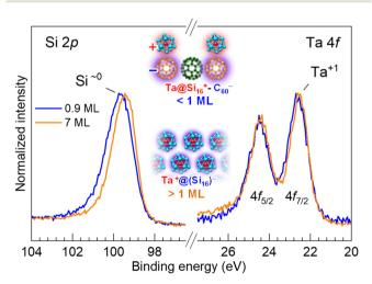
Fig. 5 Normalized XPS spectra of the thin (0.9 ML) and thick (7 ML) Ta@Si<sub>16</sub> SA films on a C<sub>60</sub> substrate. For the thick films, the Si 2p peak becomes sharper and shifts toward a lower binding energy, while the Ta 4f peak remained unchanged, corresponding to the Ta<sup>1+</sup> charge state. This result indicates that the positive charge of Ta compensates for the negatively charged Si<sub>16</sub> cage, characterizing the Ta@Si<sub>16</sub> SA as neutral
