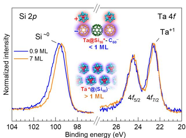
**Fig. 5** Normalized XPS spectra of the thin (0.9 ML) and thick (7 ML) Ta@Si<sub>16</sub> SA films on a C<sub>60</sub> substrate. For the thick films, the Si 2p peak becomes sharper and shifts toward a lower binding energy, while the Ta 4f peak remained unchanged, corresponding to the Ta<sup>1+</sup> charge state. This result indicates that the positive charge of Ta compensates for the negatively charged Si<sub>16</sub> cage, characterizing the Ta@Si<sub>16</sub> SA as neutral overall.
