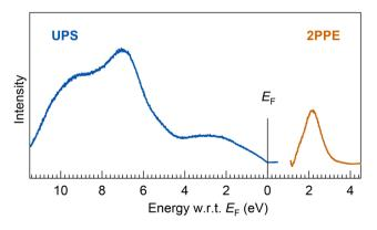
Fig. 7 (bottom) UPS and 2PPE spectra of a thick Ta@Si<sub>16</sub> SA film (7 MLs). The energy onset at  $E_{\rm F}$  in the UPS spectrum indicates the ohmic electronic conduction of the Ta@Si<sub>16</sub> SA film. The broad valence and conduction band features,  $E_{\rm F}-2.6$  eV, -7.0 eV, and -9.6 eV in UPS and  $E_{\rm F}+2.1$  eV in 2PPE, are observed. The experimental results are compared with DFT calculations for the geometric isomer of neutral species and cations, as shown ESI Fig. S8.†
