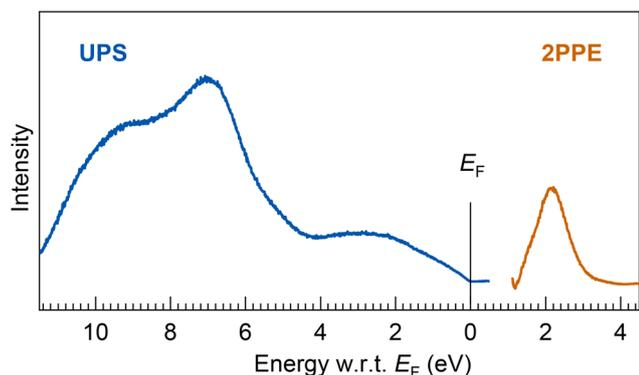
Fig. 7 (bottom) UPS and 2PPE spectra of a thick Ta@Si<sub>16</sub> SA film (7 MLs). The energy onset at  $E_F$  in the UPS spectrum indicates the ohmic electronic conduction of the Ta@Si<sub>16</sub> SA film. The broad valence and conduction band features,  $E_F - 2.6$  eV,  $-7.0$  eV, and  $-9.6$  eV in UPS and  $E_F + 2.1$  eV in 2PPE, are observed. The experimental results are compared with DFT calculations for the geometric isomer of neutral species and cations, as shown ESI Fig. S8.†
