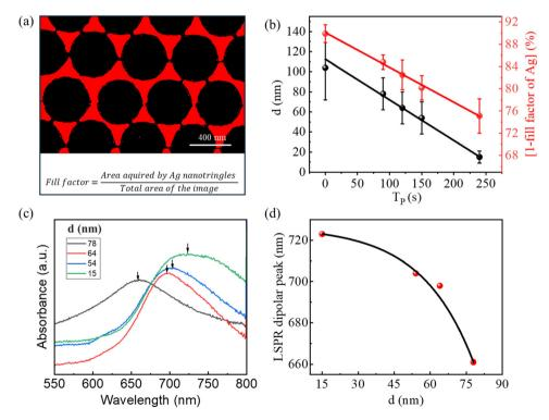
Fig. 2 (a) Ag fill factor (FF) calculation from FESEM image. (b) Average nanogap 'd' and FF variation (shown as 1 - FF) with OPT time ( $T_P$ ), (c) absorption spectra of Ag superlattice structures prepared by following  $T_p$  of 90, 120, 150, and 240 s. (d) Variation of the corresponding LSPR dipolar peak with the nanogap.
