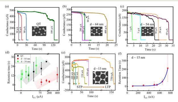
Fig. 4 Memory retention and STP to LTP transition as a function of  $I_{CC}$  for devices having (a) QT structure, (b)  $d \sim 64$  nm (c)  $d \sim 54$  nm. Retention time variation as a function of  $I_{CC}$  for (d) QT structure,  $d \sim 64$  nm, and  $d \sim 54$  nm. (e) STP to LTP transition of conductance at low  $I_{CC}$  (nA) of  $d \sim 64$  nm. 15 nm device and its (f) retention time versus  $I_{CC}$  plot.
