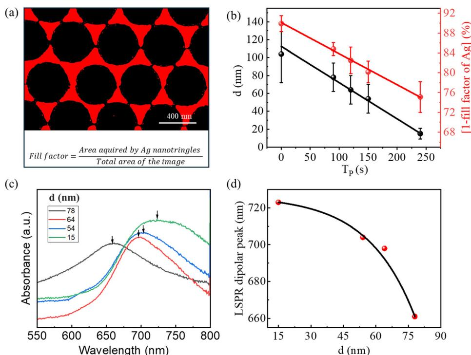
**Fig. 2** (a) Ag fill factor (FF) calculation from FESEM image. (b) Average nanogap ' $d$ ' and FF variation (shown as  $1 - FF$ ) with OPT time ( $T_p$ ), (c) absorption spectra of Ag superlattice structures prepared by following  $T_p$  of 90, 120, 150, and 240 s. (d) Variation of the corresponding LSPR dipolar peak with the nanogap.
