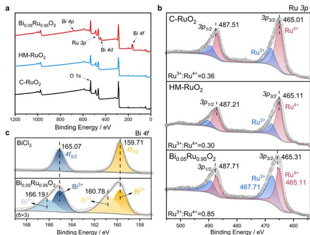
**Fig. 2** XPS analysis of the  $\text{Bi}_{0.05}\text{Ru}_{0.95}\text{O}_2$  sample. (a) XPS survey spectra of  $\text{Bi}_{0.05}\text{Ru}_{0.95}\text{O}_2$ , HM-RuO<sub>2</sub> and C-RuO<sub>2</sub>. (b) Ru 3p XPS spectra of  $\text{Bi}_{0.05}\text{Ru}_{0.95}\text{O}_2$ , HM-RuO<sub>2</sub> and C-RuO<sub>2</sub>. (c) Bi 4f XPS spectra of  $\text{Bi}_{0.05}\text{Ru}_{0.95}\text{O}_2$  and BiCl<sub>3</sub>.
