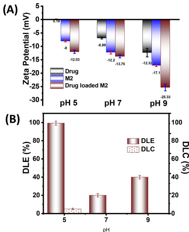
**Fig. 6** (A) Zeta potential of ciprofloxacin showing the drug in a cationic form (positively charged) at acidic pH and in anionic form (negatively charged) at basic pH along with M2 and the drug-loaded M2 microgel. (B) Drug-loading content and efficiency at different pHs.
