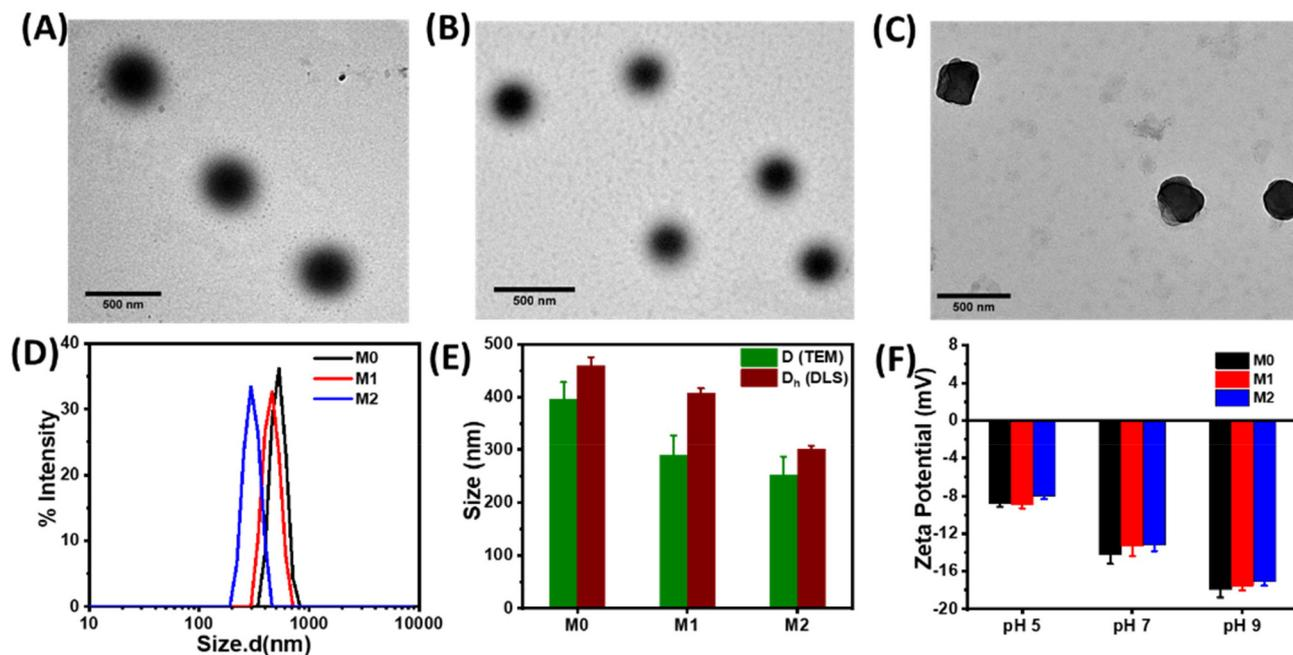
Fig. 1 TEM images of the microgels (A) M0, (B) M1, and (C) M2 drop-cast at 50 °C. (D) DLS data for the percentage intensity distribution of the microgels at 60 °C and (E) comparison of the sizes obtained from the TEM and DLS data. (F) Zeta potential of the microgels at different pHs. Sample concentration = 0.5 mg mL<sup>-1</sup>. TEM and DLS data were recorded at pH 7.
