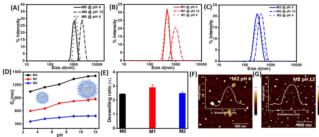
**Fig. 3** (A–C) DLS intensity data showing pH-induced reversible swelling/deswelling of the microgels **M0**, **M1**, and **M2**. (D) Variation in the hydrodynamic diameter ( $D_h$ ) of the microgels as a function of pH, showing their swollen and collapsed states. Sample concentration = 0.5 mg mL<sup>–1</sup>,  $T$  = 25 °C. (E) Histogram showing the pH-induced de/swelling factors for the microgels. (F–G) AFM height images of the **M2** microgels at pH 4 and 12, respectively.
