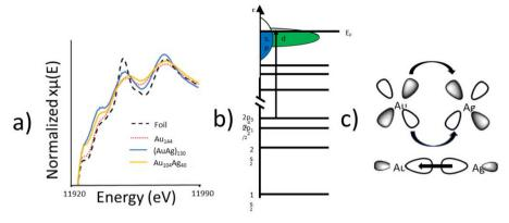
Fig. 5 Electronic properties of  $Au_{104}Ag_{40}$ . (a) Au  $L_3$ -edge XANES spectra for  $Au_{104}Ag_{40}$  alongside metallic foil reference,  $Au_{144}$ , and  $(AuAg)_{130}$ . (b) Energy diagram illustrating the Au  $L_3$ -edge electronic transition. (c) Schematic showing the electron transfer involved in the alloy interaction between Au and Aq atoms. Au donates d-electron density to Aq and receives s/p-electron density from Aq.
