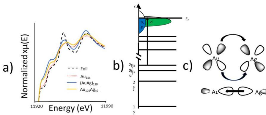
**Fig. 5** Electronic properties of  $\text{Au}_{104}\text{Ag}_{40}$ . (a) Au  $L_3$ -edge XANES spectra for  $\text{Au}_{104}\text{Ag}_{40}$  alongside metallic foil reference,  $\text{Au}_{144}$ , and  $(\text{AuAg})_{130}$ . (b) Energy diagram illustrating the Au  $L_3$ -edge electronic transition. (c) Schematic showing the electron transfer involved in the alloy interaction between Au and Ag atoms. Au donates d-electron density to Ag and receives s/p-electron density from Ag.
