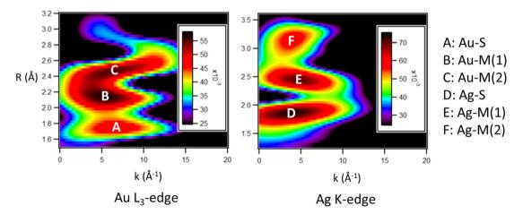
Fig. 1 WT-EXAFS plots for  $Au_{104}Ag_{40}$ . Intense features are labelled according to the bond types they represent. In the  $Au\ L_3$ -edge spectra: feature  $Au\ L_3$ -edge spectra: feature represents Au-S, feature B represents the shorter distance Au-M, and feature C represents the longer distance Au-M. In the Aq K-edge: feature D represents Ag-S, feature E represents the shorter distance Ag-M, and feature F represents the longer distance Ag-M.
