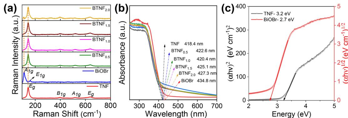
Fig. 8 (a) Raman spectroscopy analysis, (b) UV-vis diffuse reflectance spectra, and (c) corresponding band gap energy calculated using the Tauc plot of pristine  $\text{TiO}_2$  nanofiber (TNF); BiOBr; and heterojunctions of  $\text{BTNF}_{0.5}$ ,  $\text{BTNF}_{1.0}$ ,  $\text{BTNF}_{1.5}$ , and  $\text{BTNF}_{2.0}$ .
