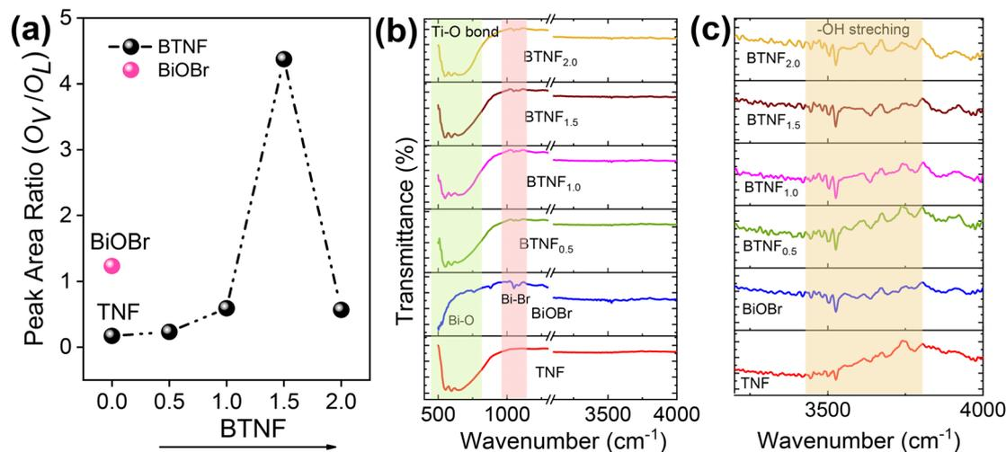
Fig. 7 (a) Peak area ratio of oxygen vacancies with lattice oxygen from XPS analysis, (b) FTIR spectrum, and (c) enlarged portion of the FTIR spectra in the 3000–4000  $\text{cm}^{-1}$  range for all the photocatalysts.
