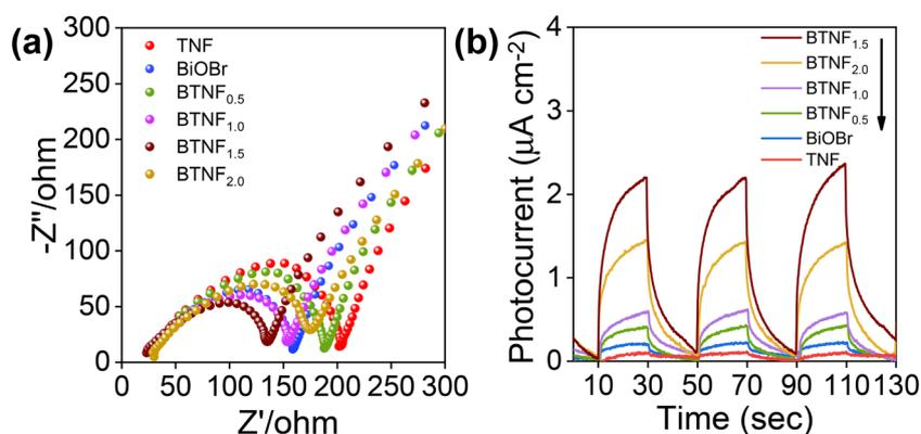
Fig. 10 (a) EIS Nyquist plot and (b) photocurrent response of pristine  $\text{TiO}_2$  nanofiber (TNF); BiOBr; and heterojunctions of  $\text{BTNF}_{0.5}$ ,  $\text{BTNF}_{1.0}$ ,  $\text{BTNF}_{1.5}$ , and  $\text{BTNF}_{2.0}$ .
