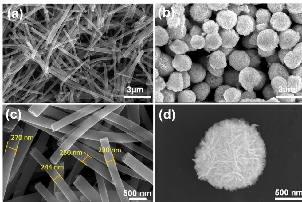
**Fig. 2** (a and b) Low-magnification image and (c and d) corresponding high-magnification image of pristine TiO<sub>2</sub> nanofiber and BiOBr microflower nanostructures.
