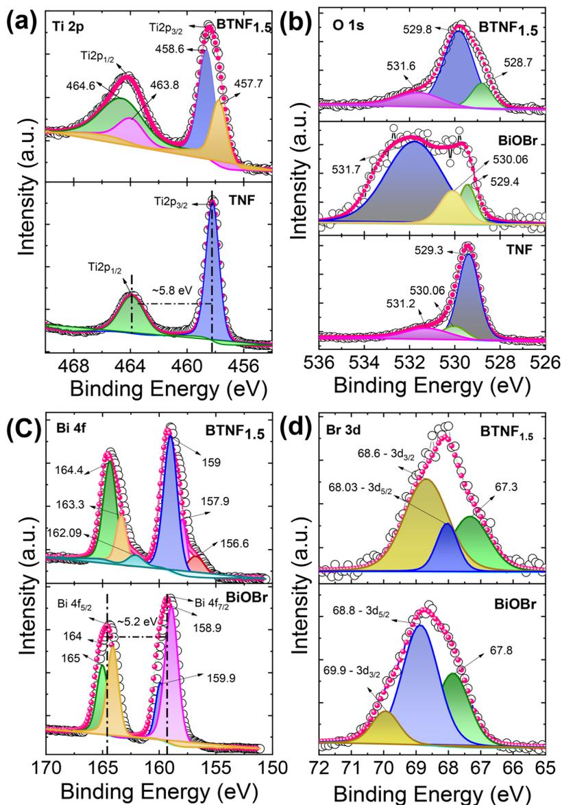
Fig. 6 High-resolution XPS spectra for elements (a) Ti 2p, (b) O 1s, (c) Bi 4f, and (d) Br 3d of BTNF<sub>1.5</sub>.
