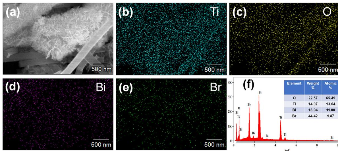
Fig. 4 (a–e) The elemental mapping images of the BTNF<sub>1.5</sub> heterojunction, and (f) corresponding atomic% in the sample.
