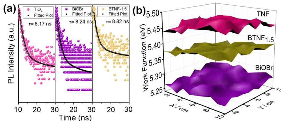
Fig. 11 (a) TCSPC kinetics and (b) SKP 3D-raster scan plot of TNF, BiOBr and BTNF<sub>1.5</sub>.
