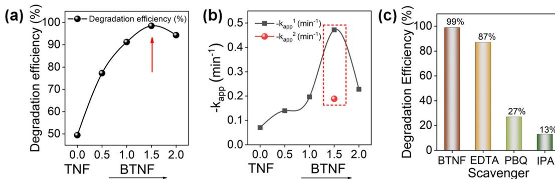
Fig. 9 (a) RhB photocatalytic degradation efficiency and (b) the relative rate constant variation with the addition of BiOBr; (c) degradation efficiency at 8 min with the addition of scavengers.
