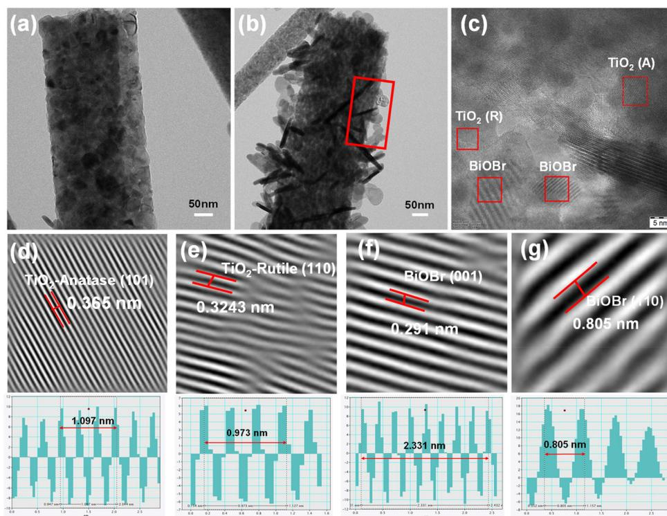
Fig. 5 (a and b) TEM images of TNF and BTNF<sub>1.5</sub> and (c) HRTEM image of BTNF<sub>1.5</sub>. (d–g) Inverse Fourier-filtered images of TiO<sub>2</sub>-anatase, rutile, and BiOBr- (001) and (110) planes with their corresponding line profiles.
