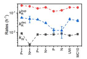
Fig. 8 Polarization buildup (dark squares and red circles) and decay (blue triangles) rates (eqn (1a)-(1c)) for the PSi NPs with different doping and oxidation. The data was acquired at 6.7 T, 1.4 K. Lines are a guide for the eye.
