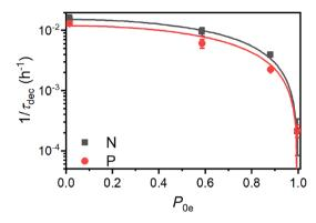
Fig. 7 The dependence of the hyperpolarization decay rate  $\tau_{\rm dec}^{-1}$  on the thermal electron polarization  $P_{0e}$  for the P and N PSi NPs. The shown experimental data was measured at (ordered with increasing  $P_{0e}$ ) 300 K, 7 T; 3.4 K, 3.4 T; 3.4 K, 7 T and 1.4 K, 6.7 T. For the fits, we assumed  $\tau_{\rm dec}^{-1} \propto 1 - P_{0e}^2$  (see main text for discussion).
