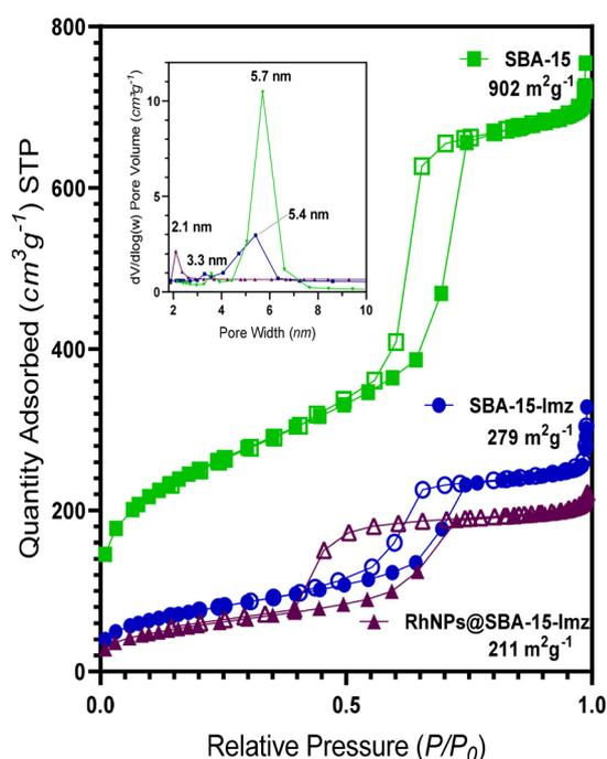
Fig. 3 Adsorption-desorption N<sub>2</sub> isotherms at 77 K of SBA-15 (green squares), SBA-15-Imz[NTf<sub>2</sub>] (blue circles) and RhNPs@SBA-15-Imz[NTf<sub>2</sub>] (purple triangles) and pore size distribution curves (inset, the pore width was estimated using the BJH model, cylindrical pores). Filled figures correspond to adsorption and hollow figures correspond to desorption.
