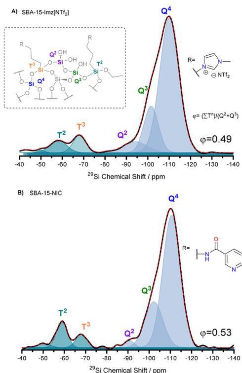
**Fig. 1**  $^{29}\text{Si}$  UDEFT-MAS NMR spectra of SBA-15-Imz[NTf<sub>2</sub>] (A) and SBA-15-NIC (B). Inset: schematic representing surface grafting possibilities for organosiloxanes on silica.
