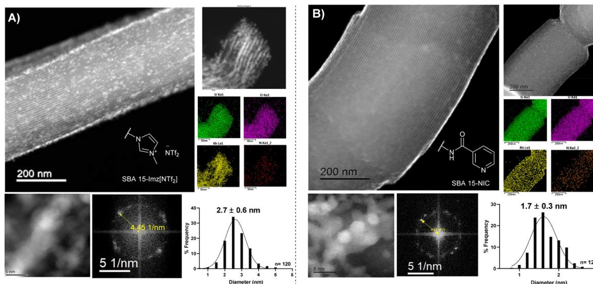
Fig. 2 HAADF-STEM micrographs, along with the corresponding FFT analysis, EDX elemental mapping, and size distribution histograms of RhNPs@SBA-15-Imz[NTf<sub>2</sub>] (A) and RhNPs@SBA-15-NIC (B).
