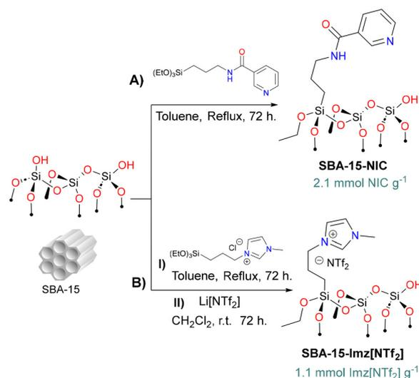
**Scheme 1** Synthesis of functionalized silica-based supports: (A) SBA-15-NIC and (B) SBA-15-Imz[NTf<sub>2</sub>].
