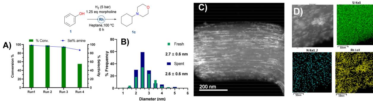
**Fig. 5** (A) Recycling of the RhNPs@SBA-15-Imz[NTf<sub>2</sub>] catalyst for the reductive amination of phenol; (B) RhNP size distribution ( $E$ ;  $n = 120$  particles) of the spent catalyst; (C) HAADF-STEM image (200 nm) and (D) EDX elemental mapping of spent RhNPs@SBA-15-Imz[NTf<sub>2</sub>].
