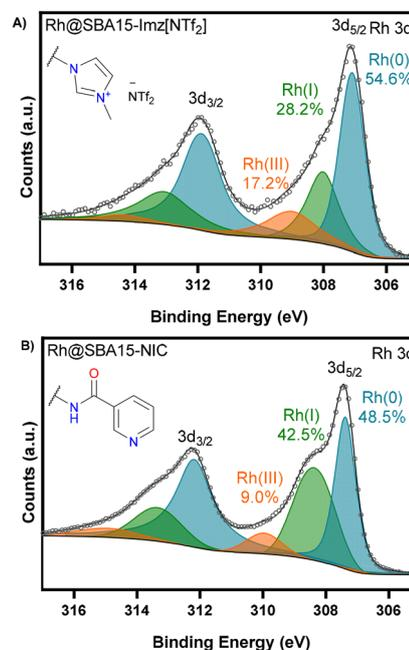
Fig. 4 High-resolution XPS analysis in the binding region corresponding to rhodium. Rh 3d for RhNPs@SBA-15-Imz[NTf<sub>2</sub>] (A) and RhNPs@SBA-15-NIC (B).
