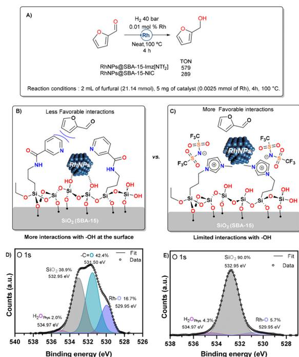
**Fig. 9** (A) RhNP performance on furfural hydrogenation under neat conditions; proposed interactions of RhNPs with (B) SBA-15-NIC and (C) SBA-15-Imz[NTf<sub>2</sub>] supports; high resolution XPS spectra of (D) RhNPs@SBA-15-NIC and (E) RhNPs@SBA-15-Imz[NTf<sub>2</sub>].
