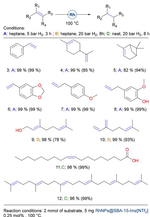
Fig. 6 RhNP catalysed hydrogenation of biomass-derived alkenes.
