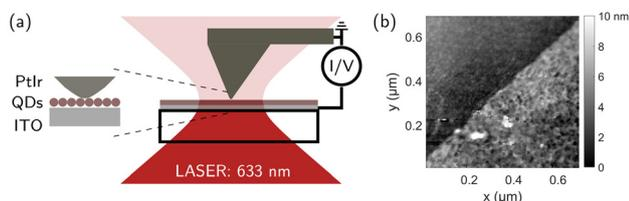
**Fig. 1** (a) Sketch of the pAFM with a PtIr tip to probe QD layers. With a grounded tip, the bias is applied to the sample and the photocurrent is measured with an  $I/V$  amplifier. (b) Peak force tapping AFM image of a PbS/MAPbI<sub>3</sub> QD layer edge with a measured step height of  $3.8 \pm 0.7 \text{ nm}$  (averaged along the edge).
