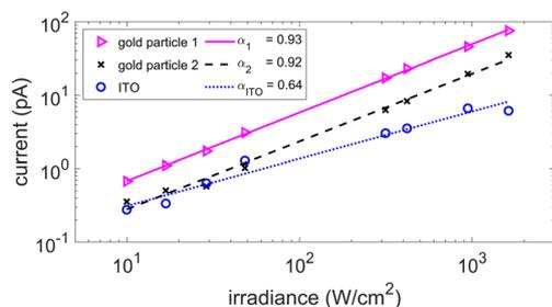
**Fig. 6** Measured irradiance-dependent currents (symbols) and power law fits (lines) for a QD monolayer on two different gold nanotriangles (black, magenta) and on ITO (blue). Contact mode with 0.6 nN setpoint force, 0.1 V bias voltage and focusing by the 10 $\times$  objective.
