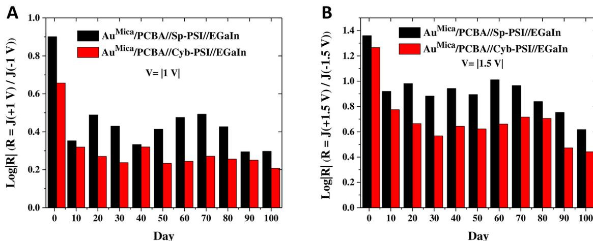
**Fig. 7** Comparison of the rectification ratios of PSI complexes (A) at  $V = |1 \text{ V}|$  and (B) at  $V = |1.5 \text{ V}|$  solid-state junctions. For both voltages, the rectification ratios of Cyb-PSI and Sp-PSI exhibit fluctuations over approximately 100 days, with a trend showing a decrease from day 1 to day 100. This decline in rectification ratios suggests a diminishing trend over the observed period.
