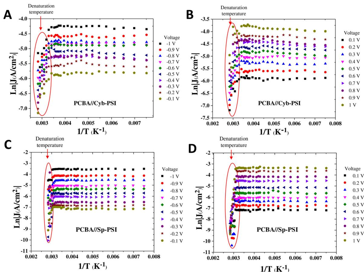
Fig. 5 Arrhenius plots of bilayer comprising of Au<sup>Mica</sup>/PCBA//Cyb-PSI//EGaIn (A–B) and Au<sup>Mica</sup>/PCBA//Sp-PSI//EGaIn junctions (C–D) between temperature ranges 133–353 K from –0.1 to –1 V (A, C) and from 0.1 to 1 V (B, D). The red ovals show the temperatures corresponding to PSI protein denaturation.
