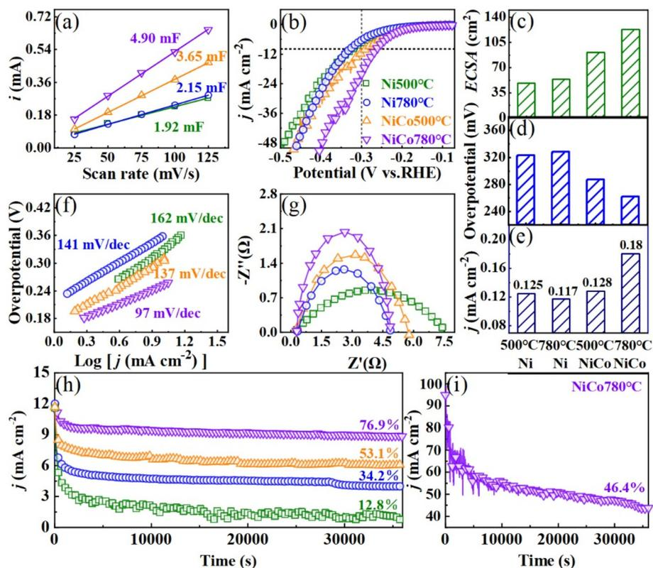
Fig. 6 (a) Electric double layer capacitance, (b) LSV curve, (c) ECSA, (d) overpotential at  $10 \text{ mA cm}^{-2}$ , (e) area activity at  $-0.3 \text{ V}$ , (f) Tafel slope, and (g) electrochemical impedance of Ni and NiCo alloy catalysts. (h) Stability test of Ni and NiCo alloy catalysts at  $10 \text{ mA cm}^{-2}$  and (i) stability test of  $L_{10}$ -NiCo alloys at  $100 \text{ mA cm}^{-2}$ .
