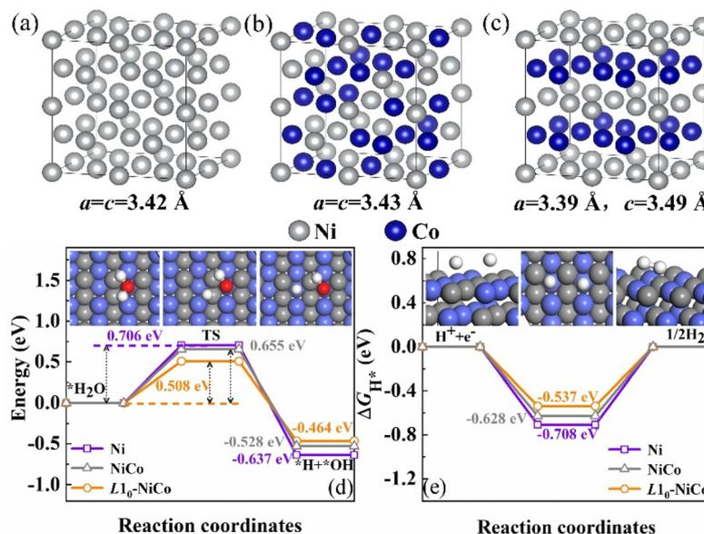
**Fig. 1** (a) Ni, (b) disordered NiCo solid solution, and (c) and ordered intermetallic  $L1_0$ -NiCo  $2 \times 2 \times 2$  supercell. (d) The energy difference of the  $\text{H}_2\text{O}$  dissociation process. (e) H adsorption Gibbs free energy diagram.
