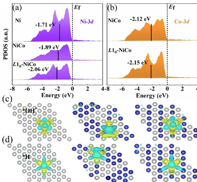
**Fig. 2** (a) The density of states and d-band center of Ni and (b) Co atoms, (c) the differential charge density diagram of \*OH<sup>-</sup> and (d) \*H of Ni, disordered NiCo solid solution and ordered intermetallic L<sub>10</sub>-NiCo.
