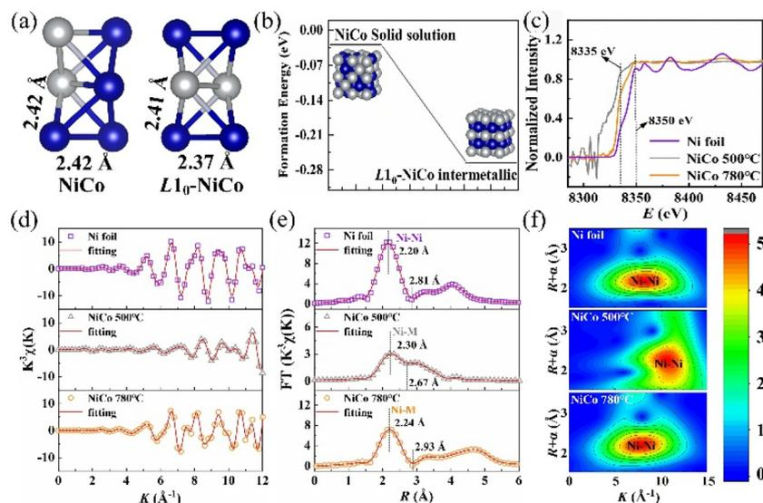
**Fig. 4** (a) Ni–Ni and Ni–Co bond length of the Ni foil and NiCo alloy. (b) The formation energy of disordered NiCo solid solution and intermetallic  $L1_0$ -NiCo. (c) Ni K-edge XANES spectrum, (d) oscillation curve of the Ni K edge XAFS  $K^2\chi(K)$ , (e) Fourier transform of Ni K-edge EXAFS spectra and (f) EXAFS wavelet transform diagram of the Ni foil and NiCo alloy.
